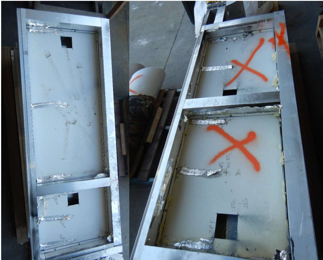
Figure 44 The unexposed face of backpan of modules 7 and 6, respectively, after sampling at the end of the test.
