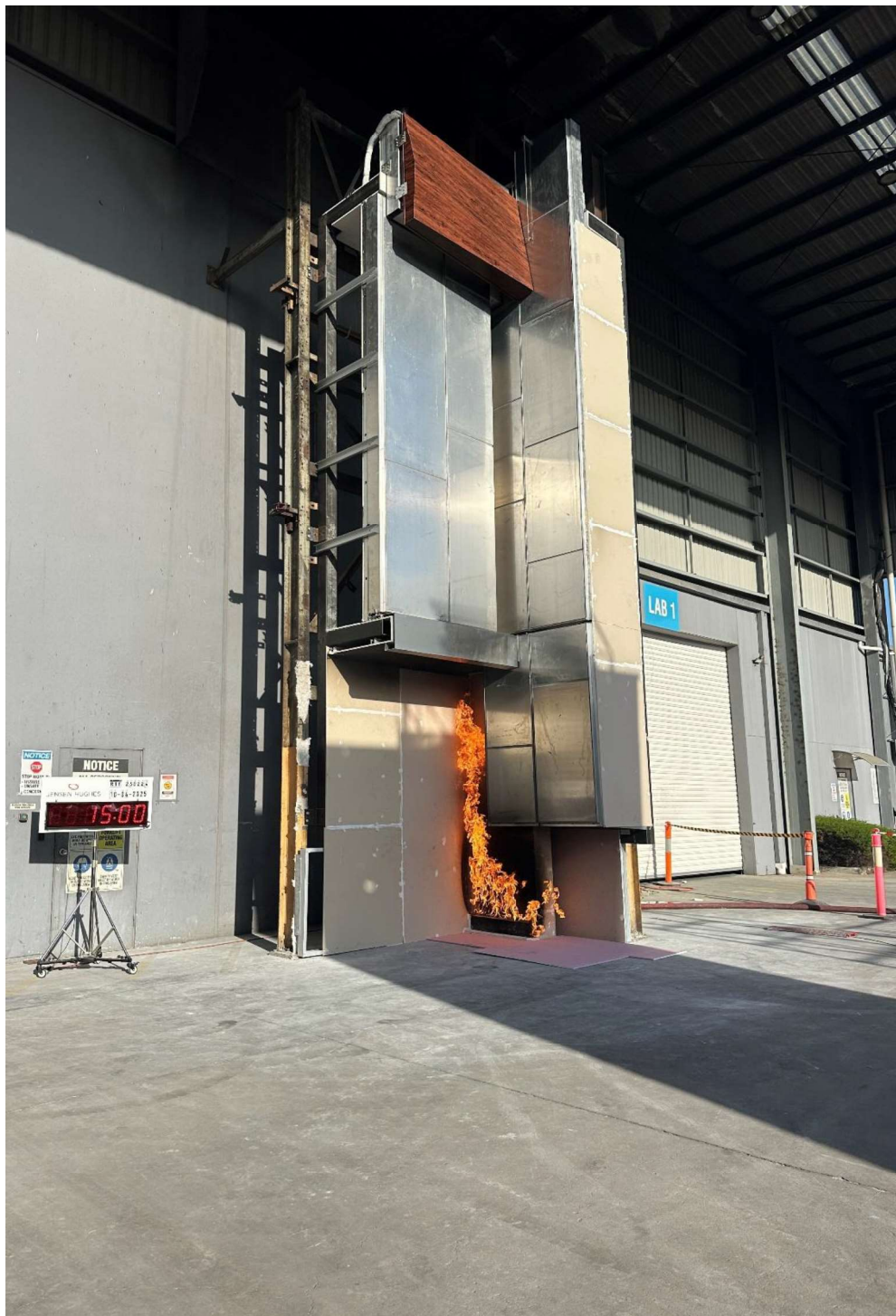
Figure 40 The specimen 15 minutes into the test, the burner was increased to 300 kW.
