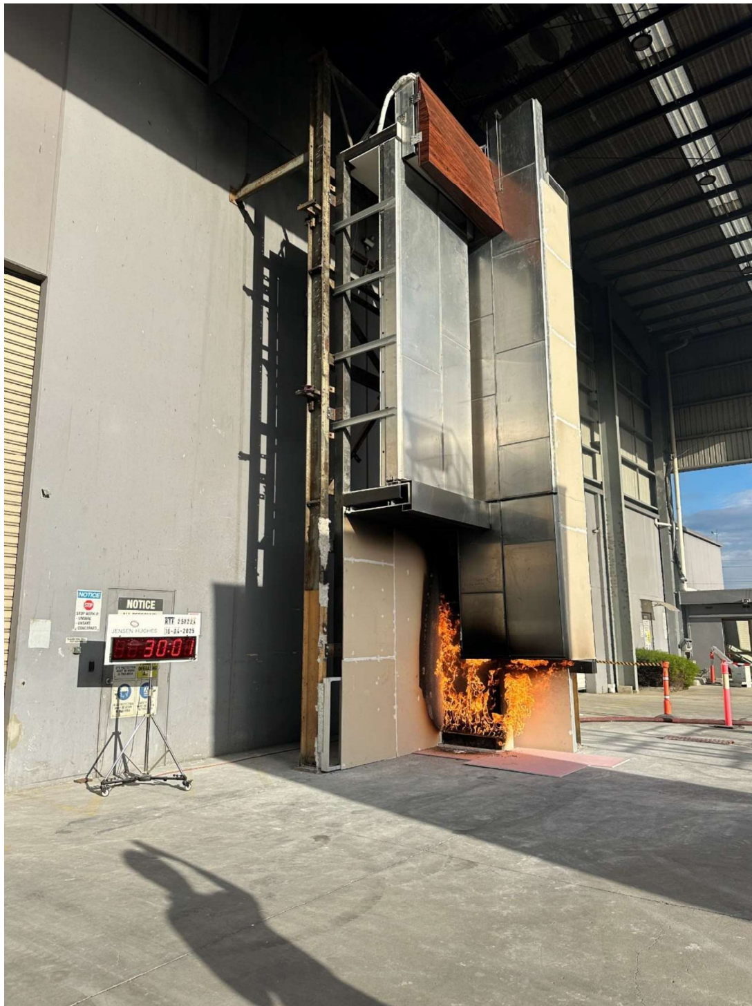
Figure 41 The specimen 30 minutes 1 second into the test – 15 minutes 1 second after the burner output was increased to 300 kW.
