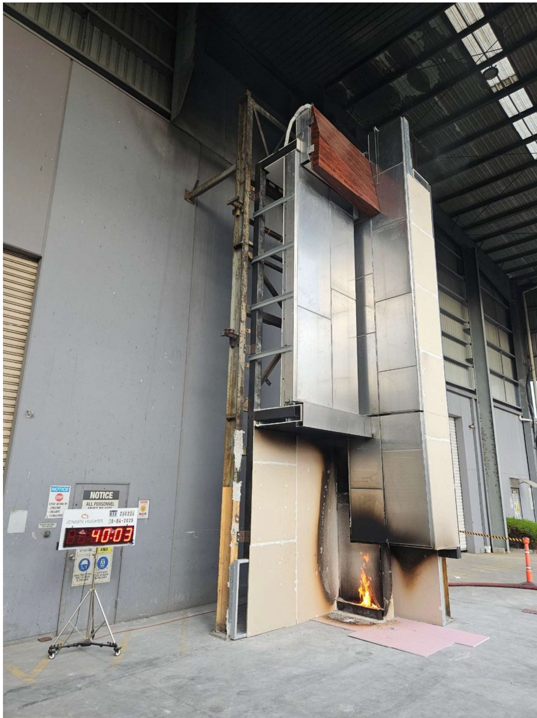
Figure 42 The specimen 40 minutes 3 seconds into the test – 3 seconds after the burner was turned off.
