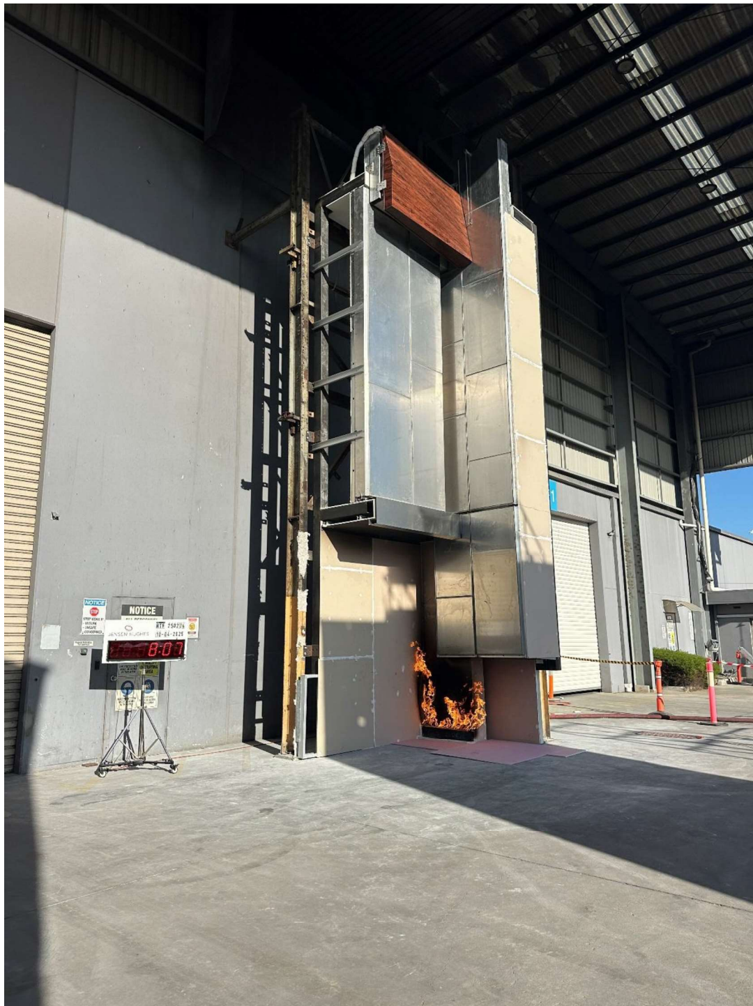
Figure 39 The specimen 8 minutes 7 seconds into the test with the burner at 100 kW.
