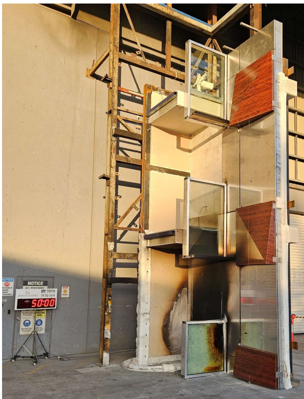
Figure 40 The specimen 50 minutes into the test – 35 minutes after the burner output was increased to 300 kW.
