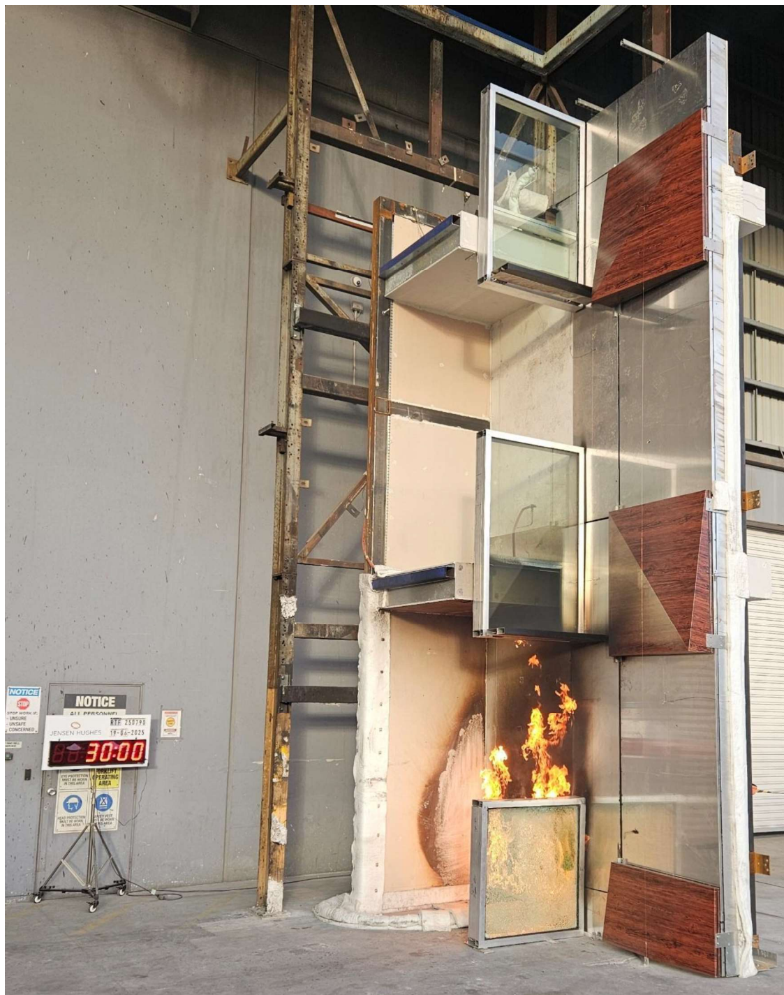
Figure 37 The specimen 30 minutes into the test – 15 minutes after the burner output was increased to 300 kW.
