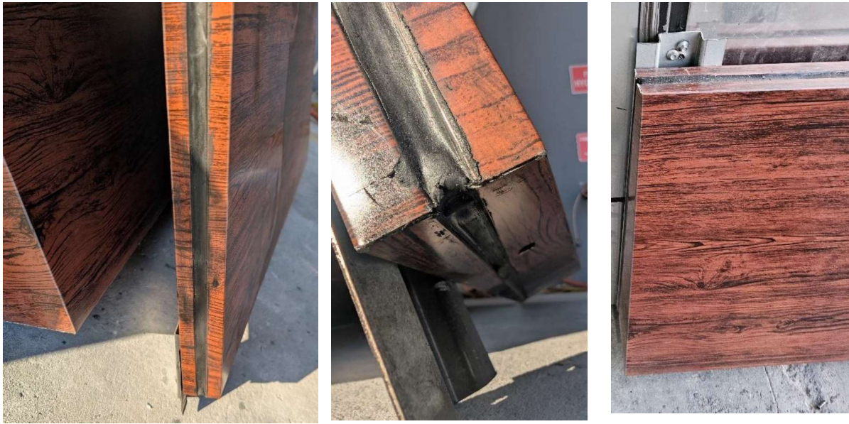
Figure 42 Post test condition of the ground level architectural module
