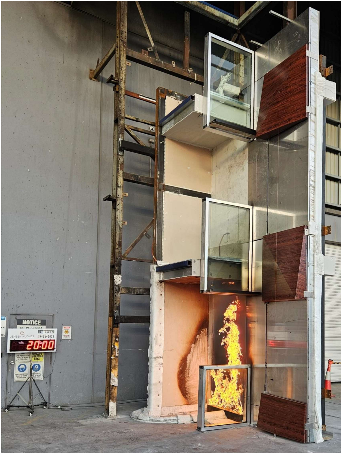
Figure 36 The specimen 20 minutes into the test – 5 minutes after the burner output was increased to 300 kW.
