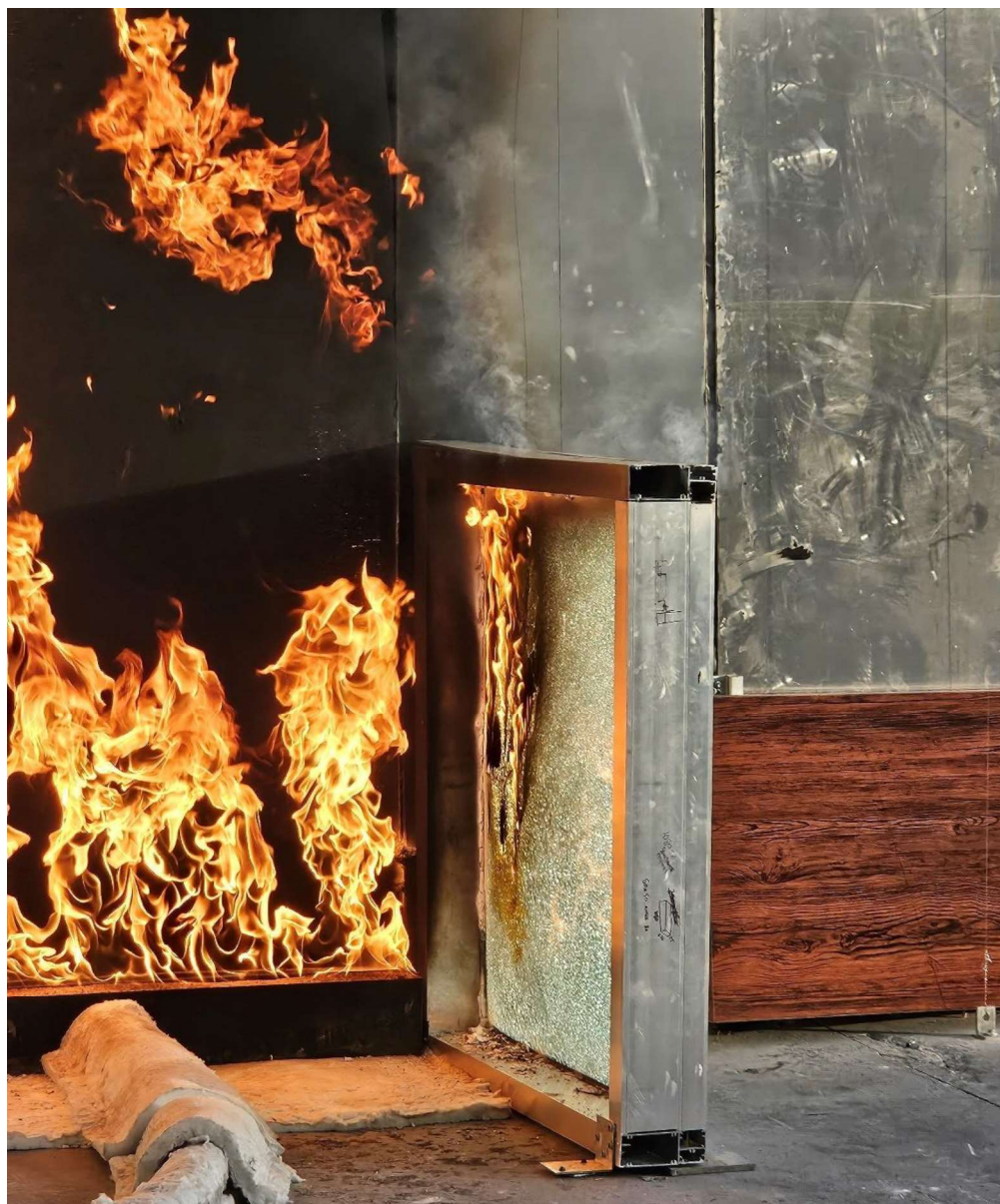
Figure 38 The specimen 31 minutes and 45 seconds into the test – flaming on sealant and glazing of the ground level balustrade.
