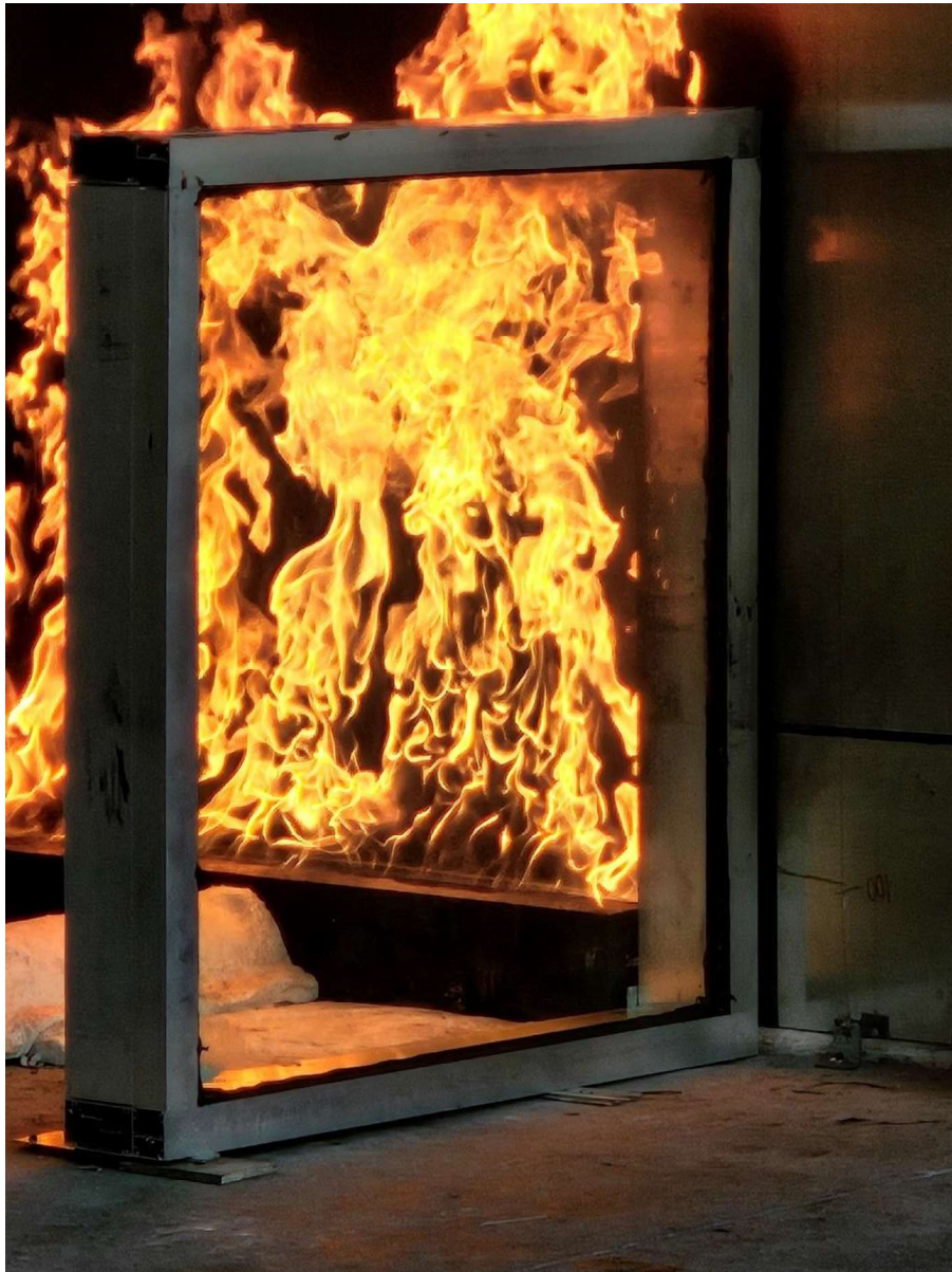
Figure 35 The specimen 19 minutes 56 seconds into the test – formation of bubbles in the PVB interlayer of glazing.
