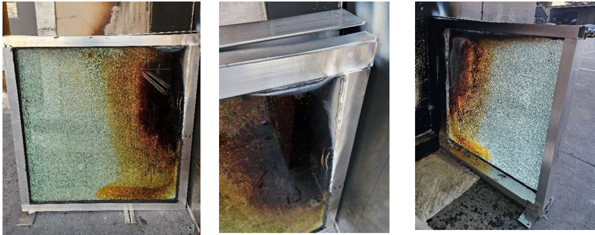
Figure 44 Post test condition of the ground level balustrade
