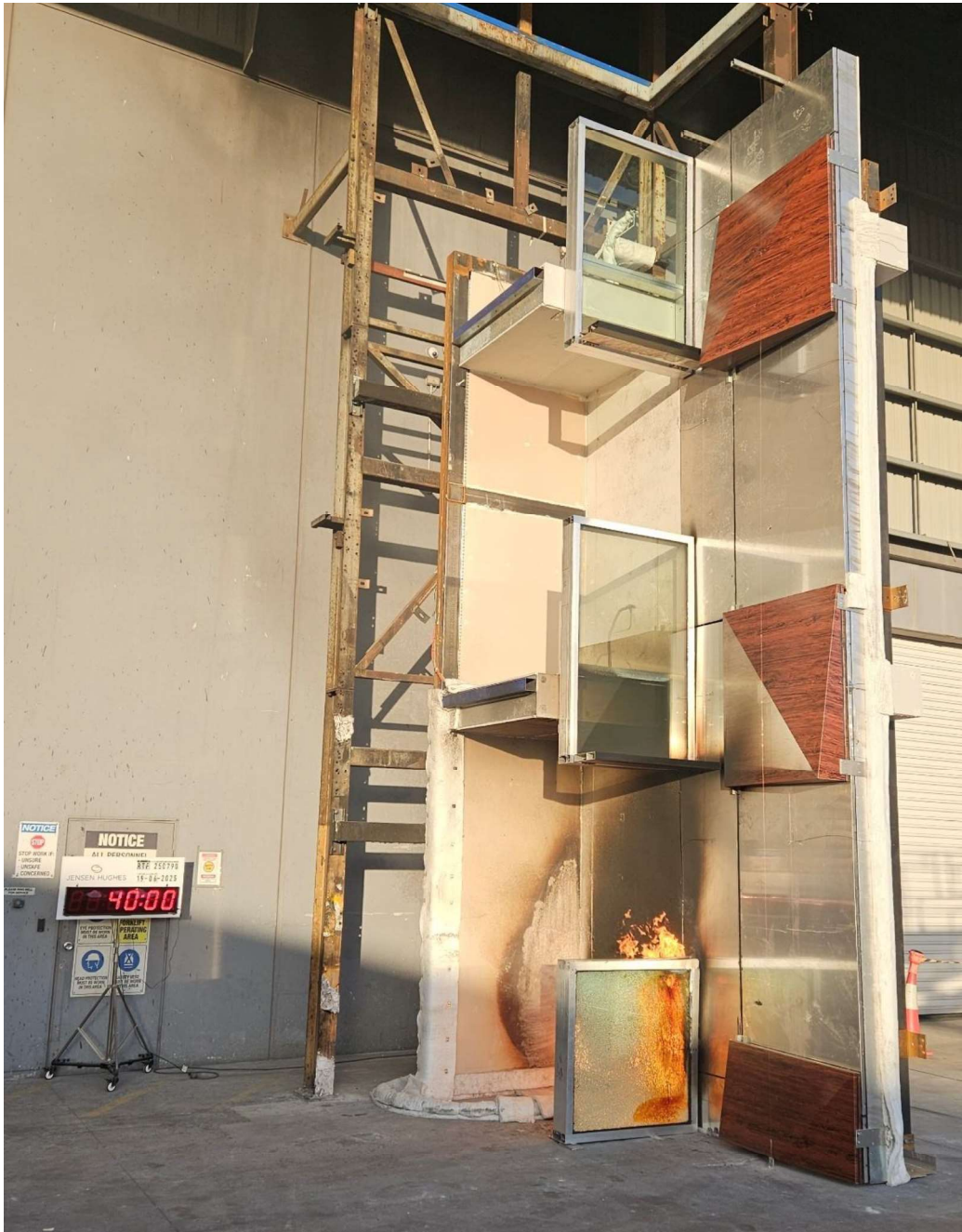
Figure 39 The specimen 40 minutes into the test – 25 minutes after the burner output was increased to 300 kW - burner was tuned off.
