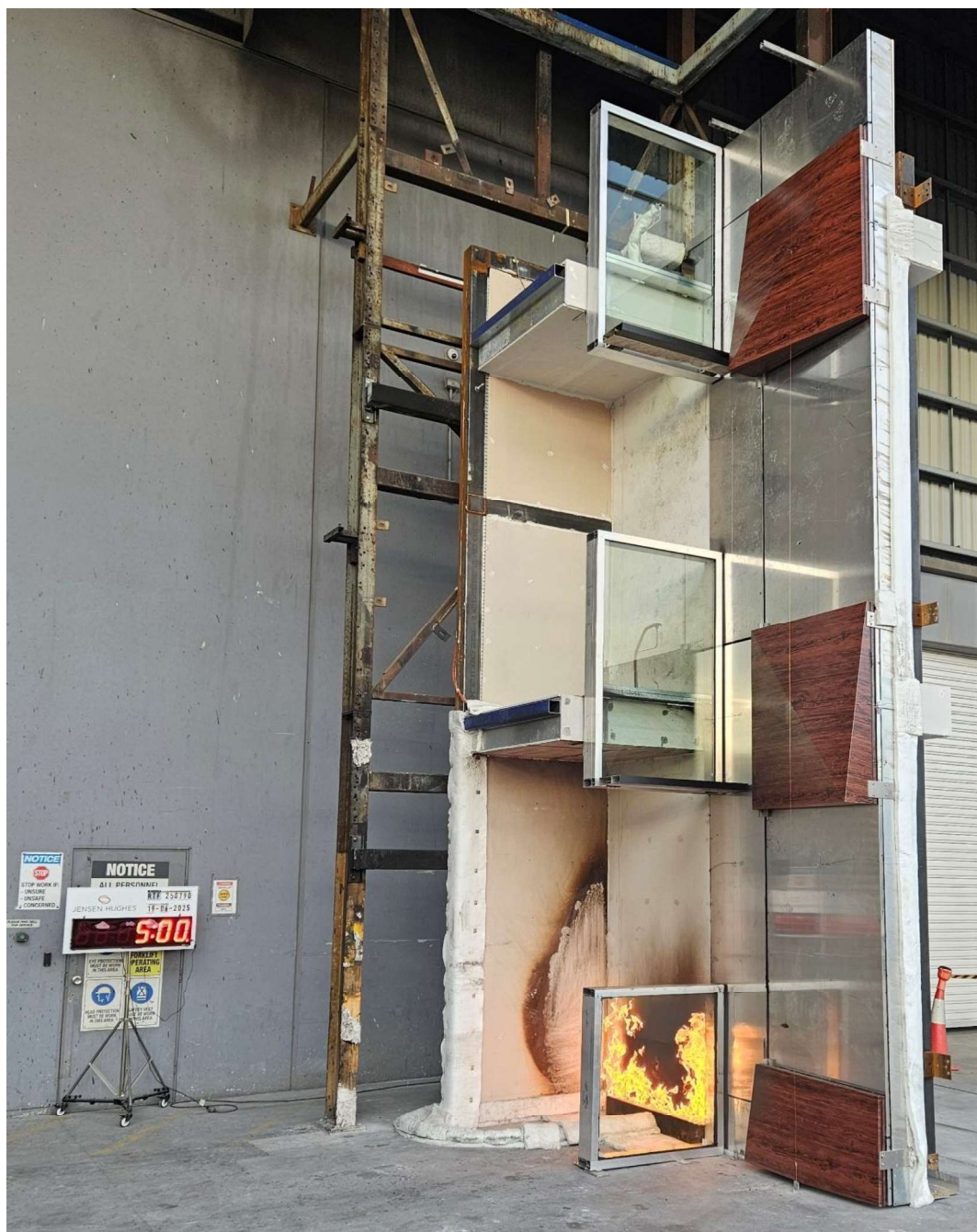
Figure 32 The specimen 5 minutes into the test with the burner at 100 kW.
