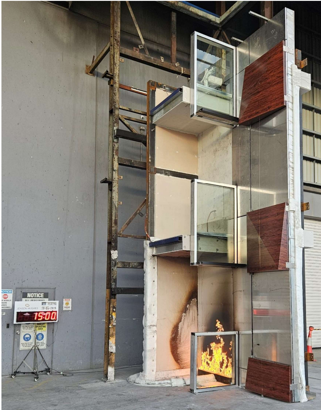
Figure 34 The specimen 15 minutes into the test – the burner output was increased to 300 kW.
