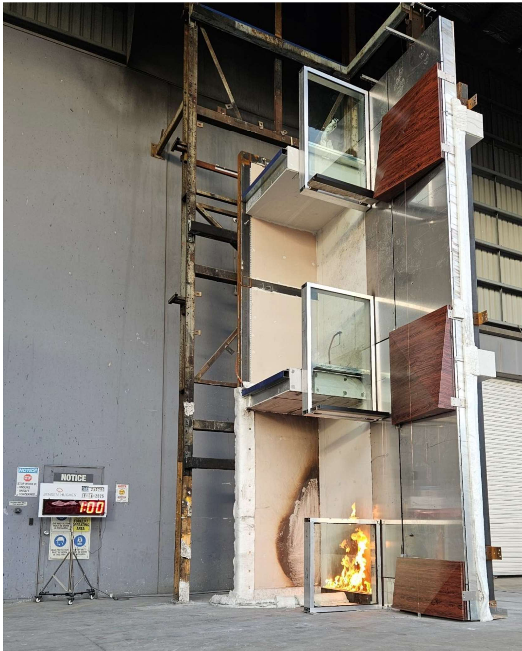
Figure 31 The specimen 1 minute into the test with the burner at 100 kW.
