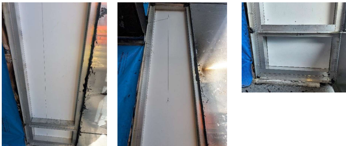
Figure 47 Post test condition of the ACP back pan.
