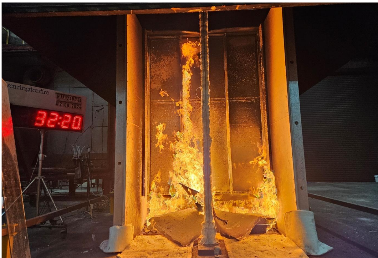
Figure 27 The specimen 32 minutes 20 seconds into the test (burner output at 300 kW)
