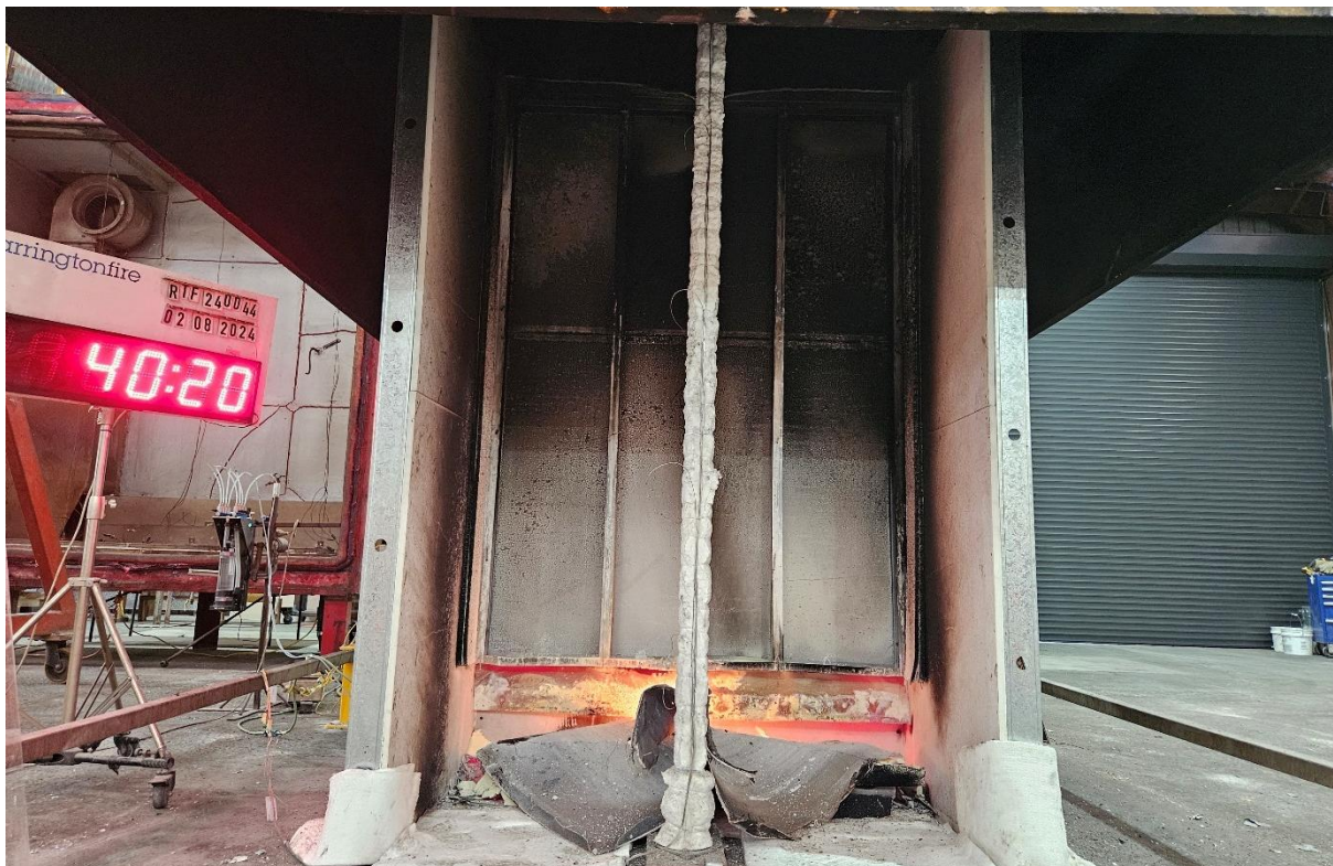
Figure 29 The specimen 40 minutes 20 seconds into the test (burner off)
