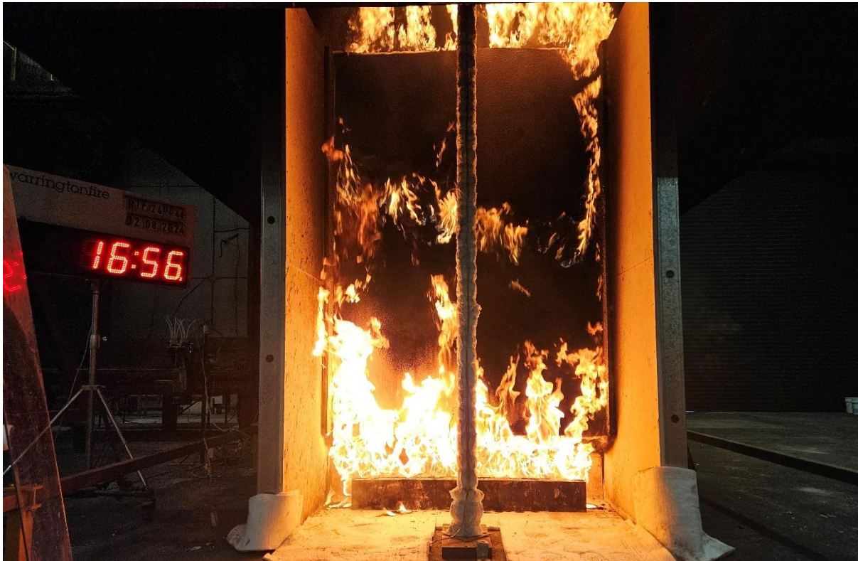
Figure 22 The specimen 16 minutes 56 seconds into the test (burner output at 300 kW)
