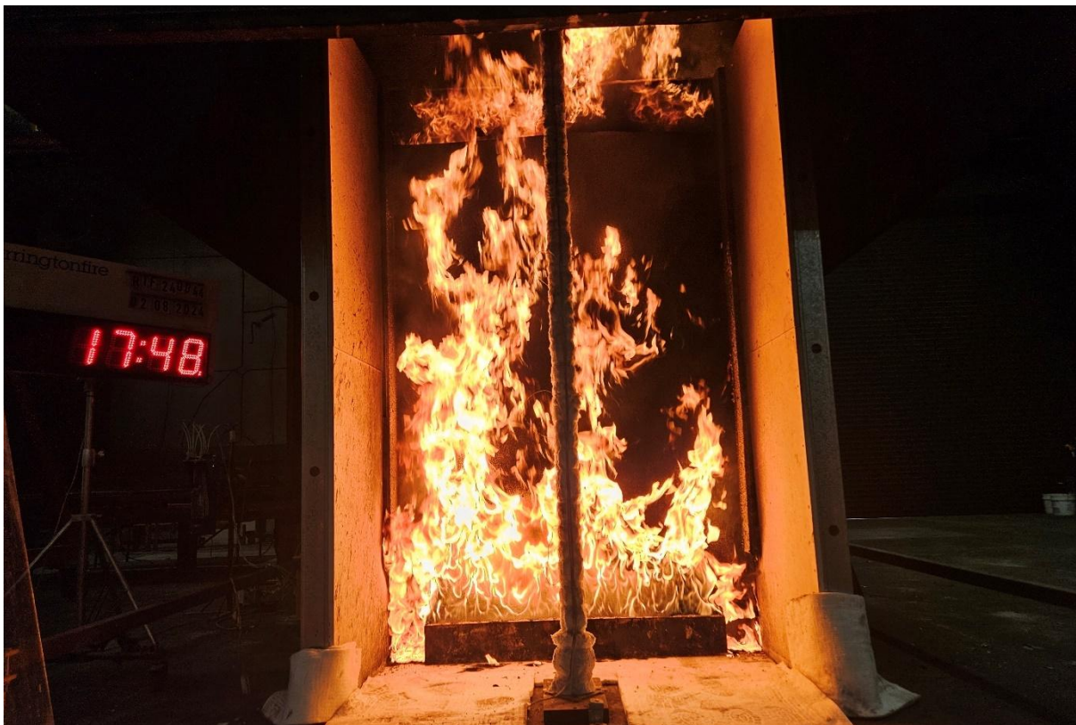
Figure 23 The specimen 17 minutes 48 seconds into the test (burner output at 300 kW)
