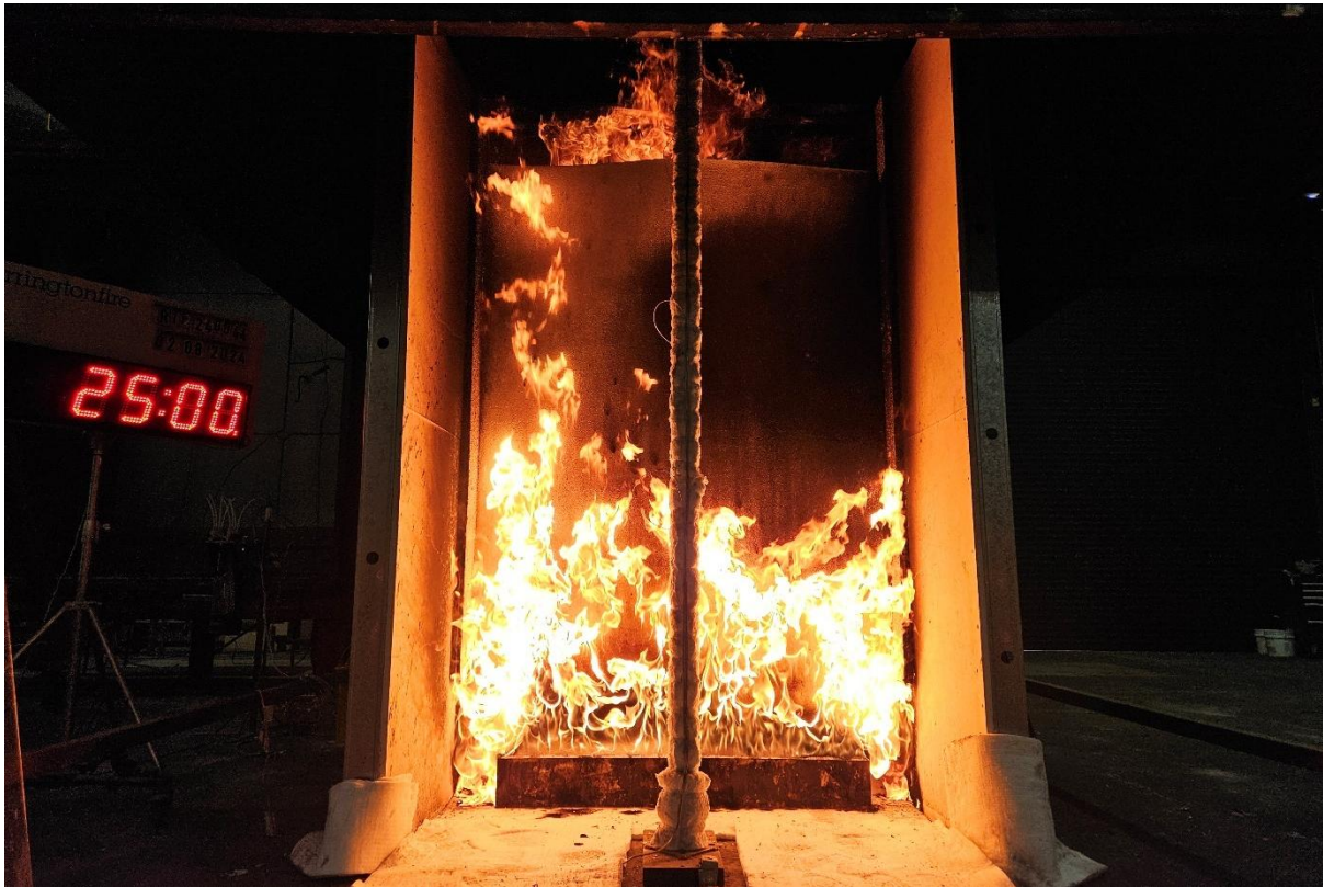
Figure 24 The specimen 25 minutes into the test (burner output at 300 kW)
