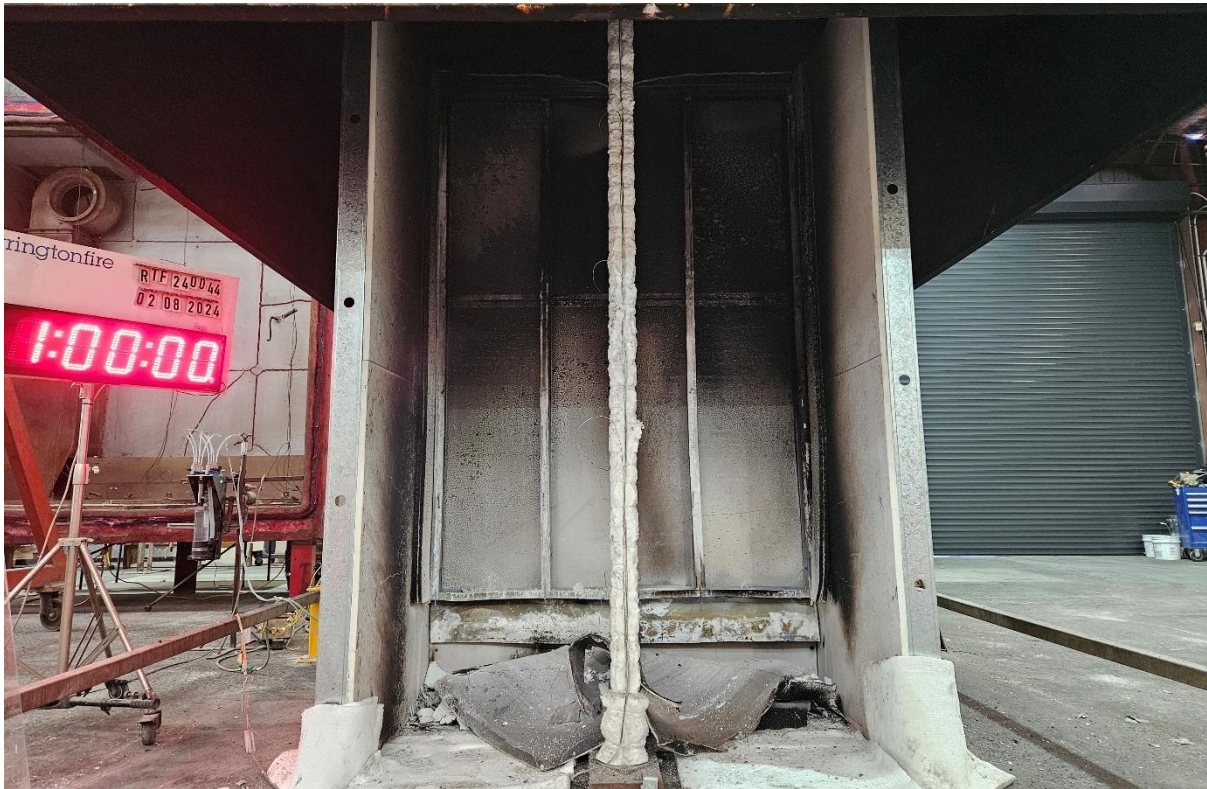
Figure 30 The specimen at end of the reaction to fire test – exposed side
