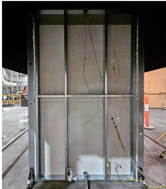
Figure 17 The specimen before the reaction to fire test – unexposed side
