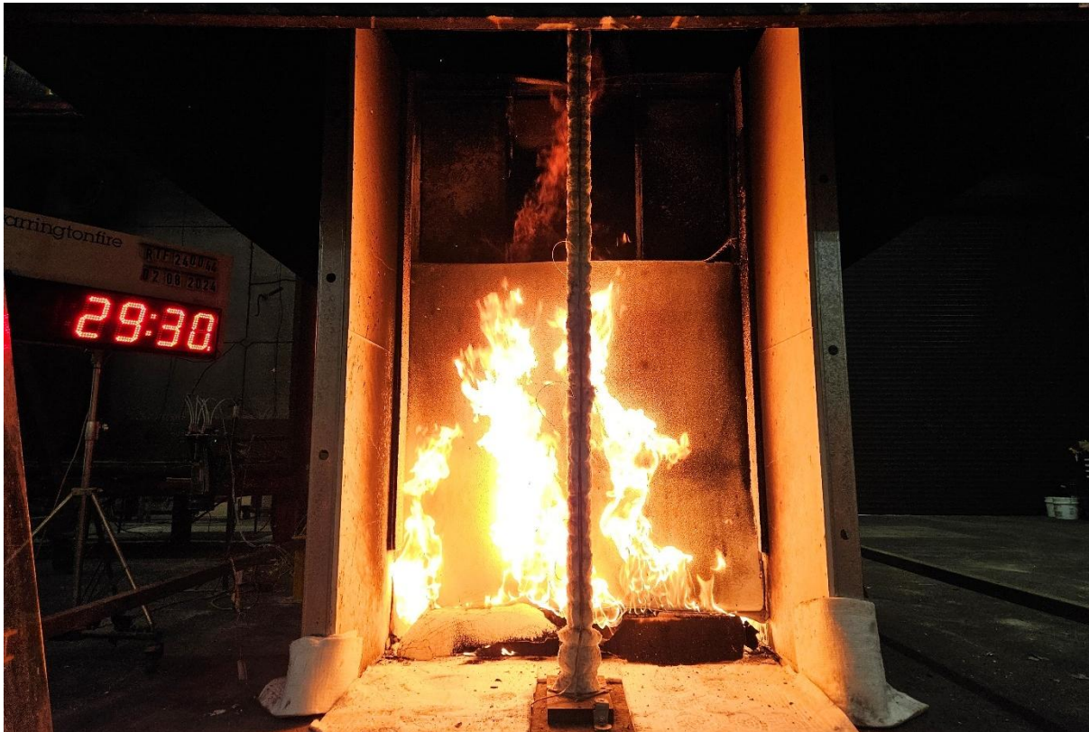
Figure 25 The specimen 29 minutes 30 seconds into the test (burner output at 300 kW)
