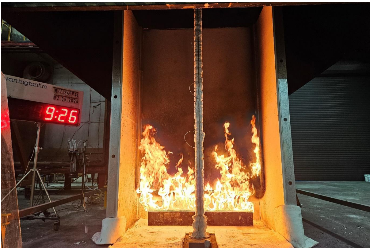
Figure 19 The specimen 9 minutes 26 seconds into the test (burner output at 100 kW)
