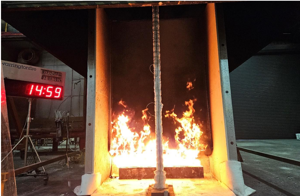
Figure 20 The specimen 14 minutes 59 seconds into the test (burner output at 100 kW)
