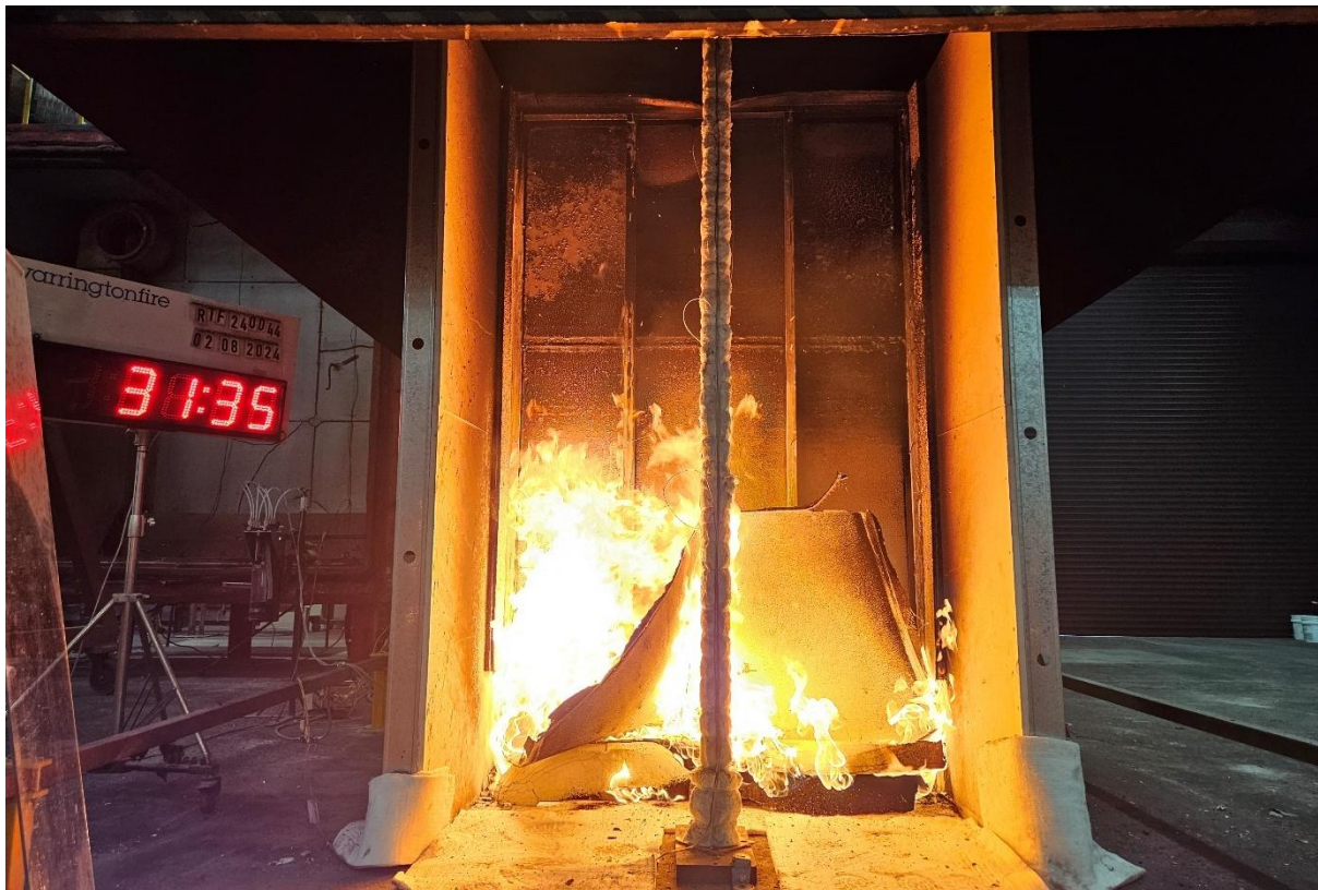
Figure 26 The specimen 31 minutes 35 seconds into the test (burner output at 300 kW)
