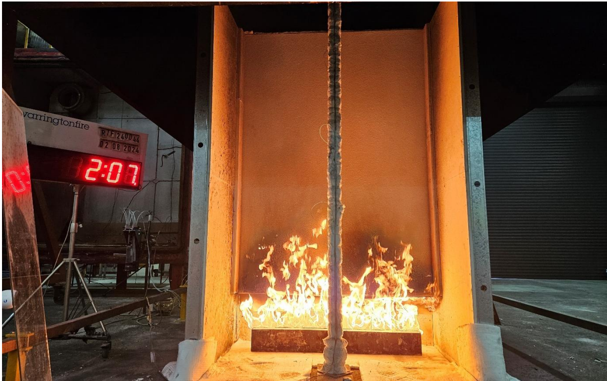
Figure 18 The specimen 2 minutes 7 seconds into the test (burner output at 100 kW)
