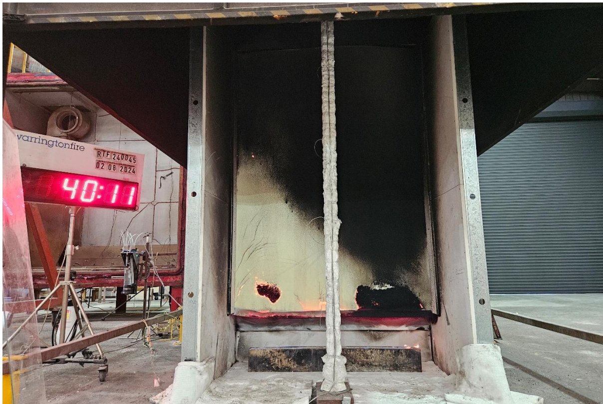
Figure 24 The specimen 40 minutes 11 seconds into the test (burner off)
