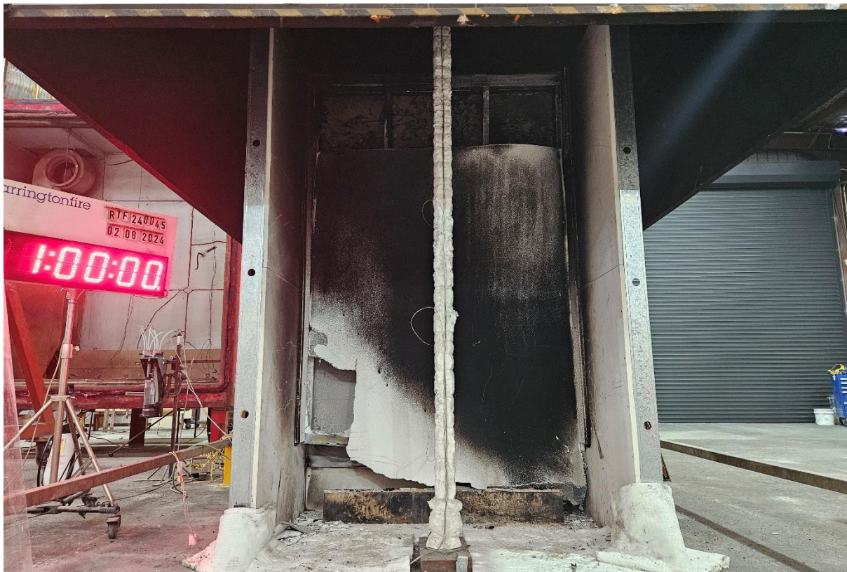
Figure 28 The specimen at end of the reaction to fire test – exposed side
