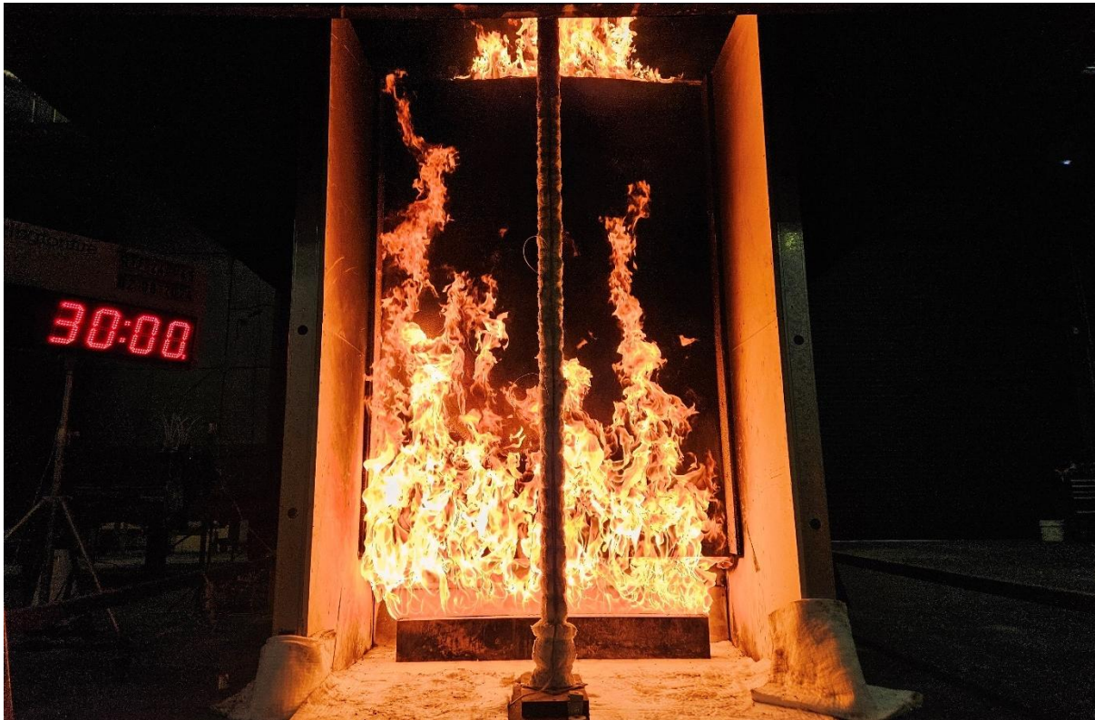
Figure 22 The specimen 30 minutes into the test (burner output at 300 kW)
