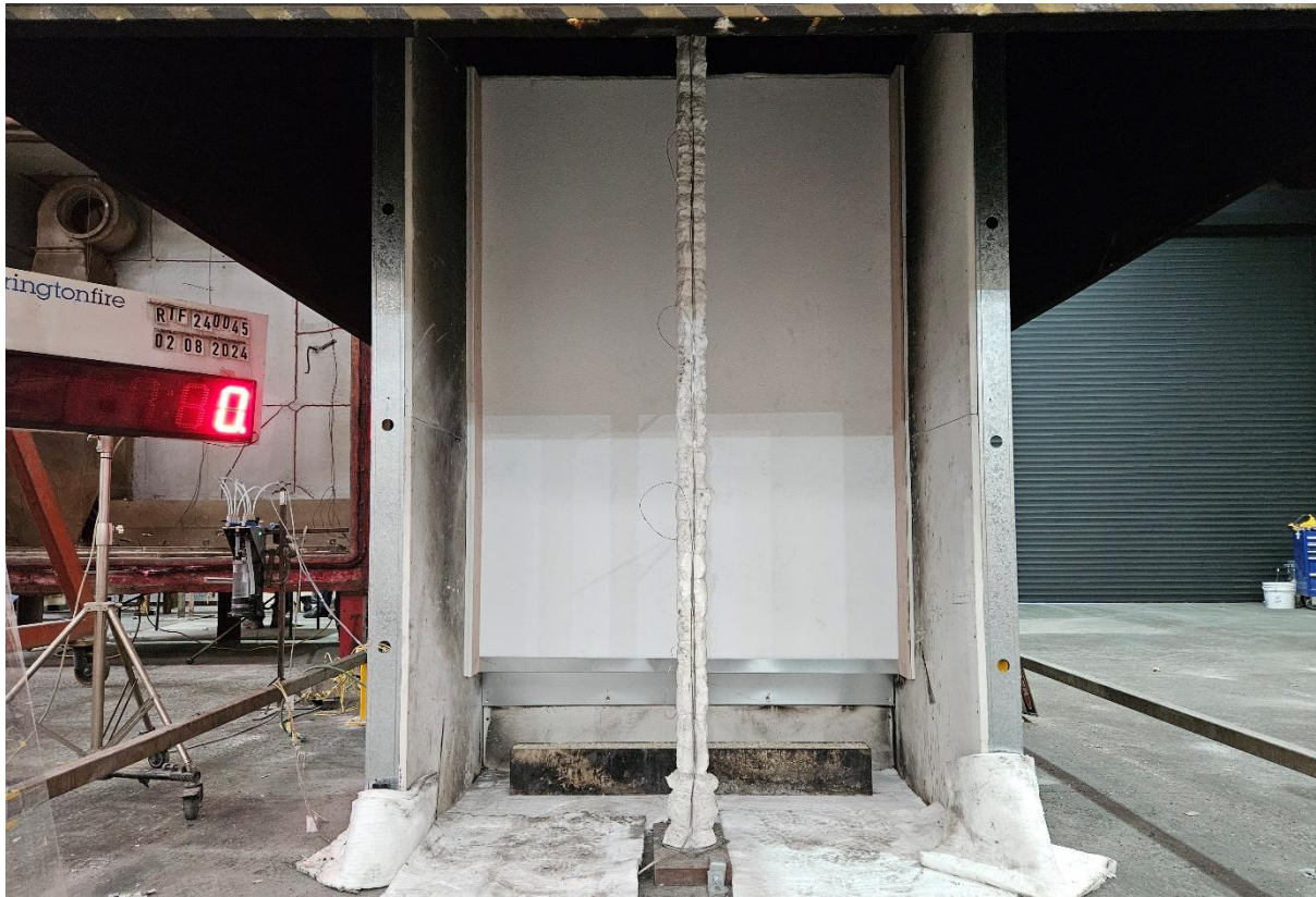
Figure 16 The specimen before the reaction to fire test – exposed side
