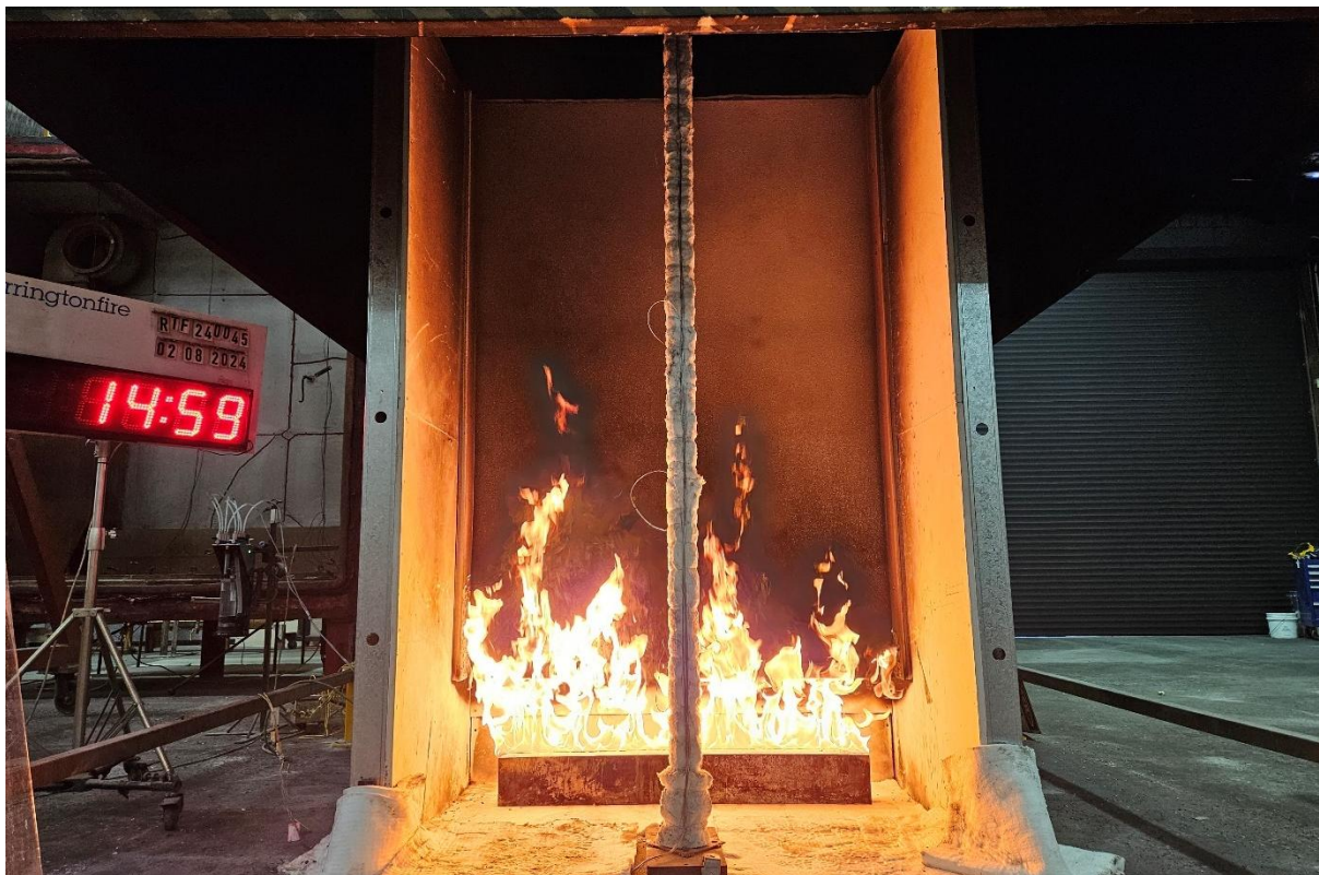
Figure 19 The specimen 14 minutes 59 seconds into the test (burner output at 100 kW)
