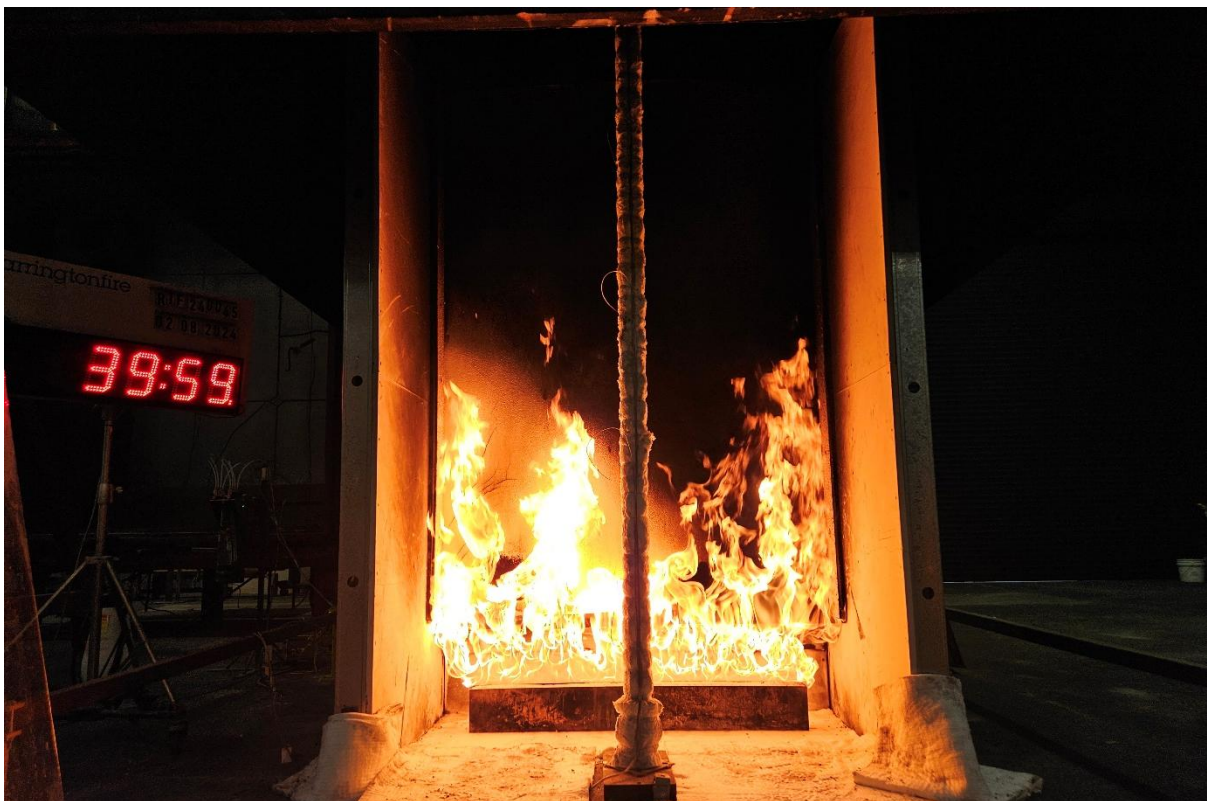
Figure 23 The specimen 39 minutes 59 seconds into the test (burner output at 300 kW)
