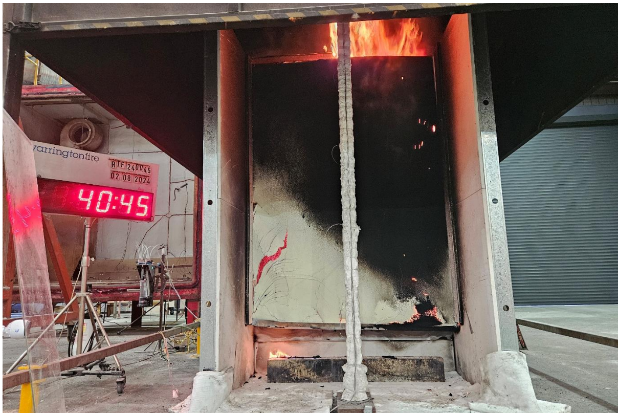
Figure 25 The specimen 40 minutes 45 seconds into the test (burner off)
