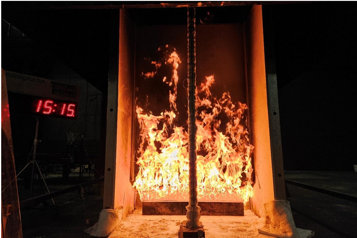
Figure 20 The specimen 15 minutes 15 seconds into the test (burner output at 300 kW)
