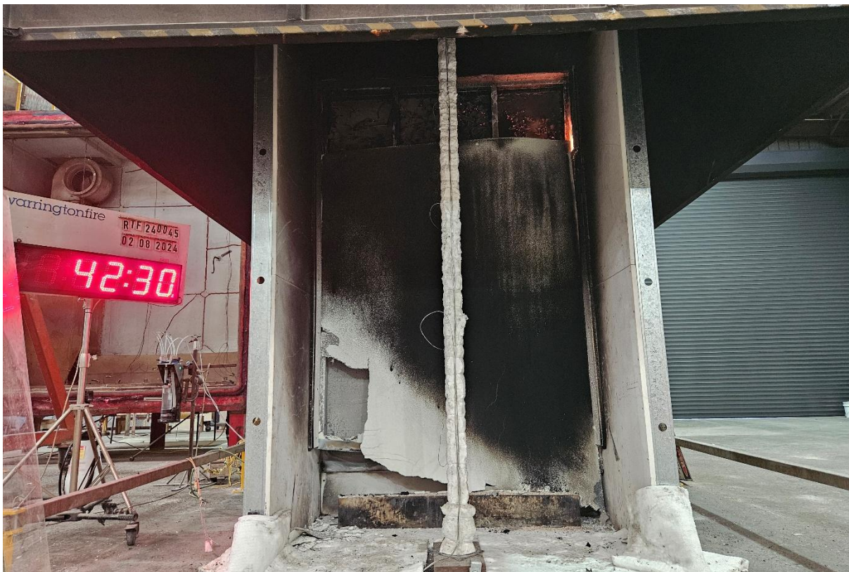
Figure 27 The specimen 42 minutes 30 seconds into the test (burner off)
