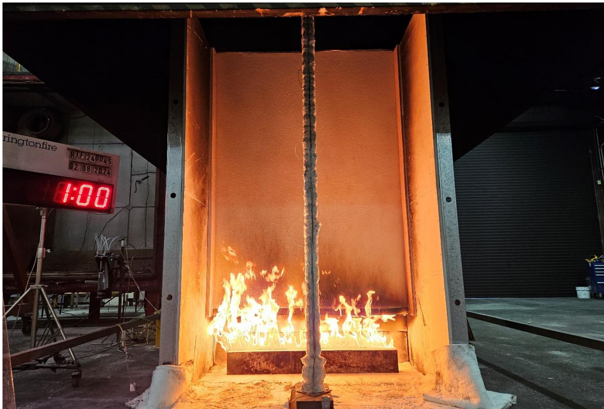
Figure 18 The specimen 1 minute into the test (burner output at 100 kW)
