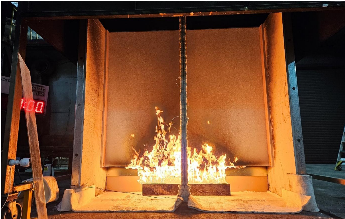
Figure 18 The specimen 3 minutes into the test (burner output at 100 kW)
