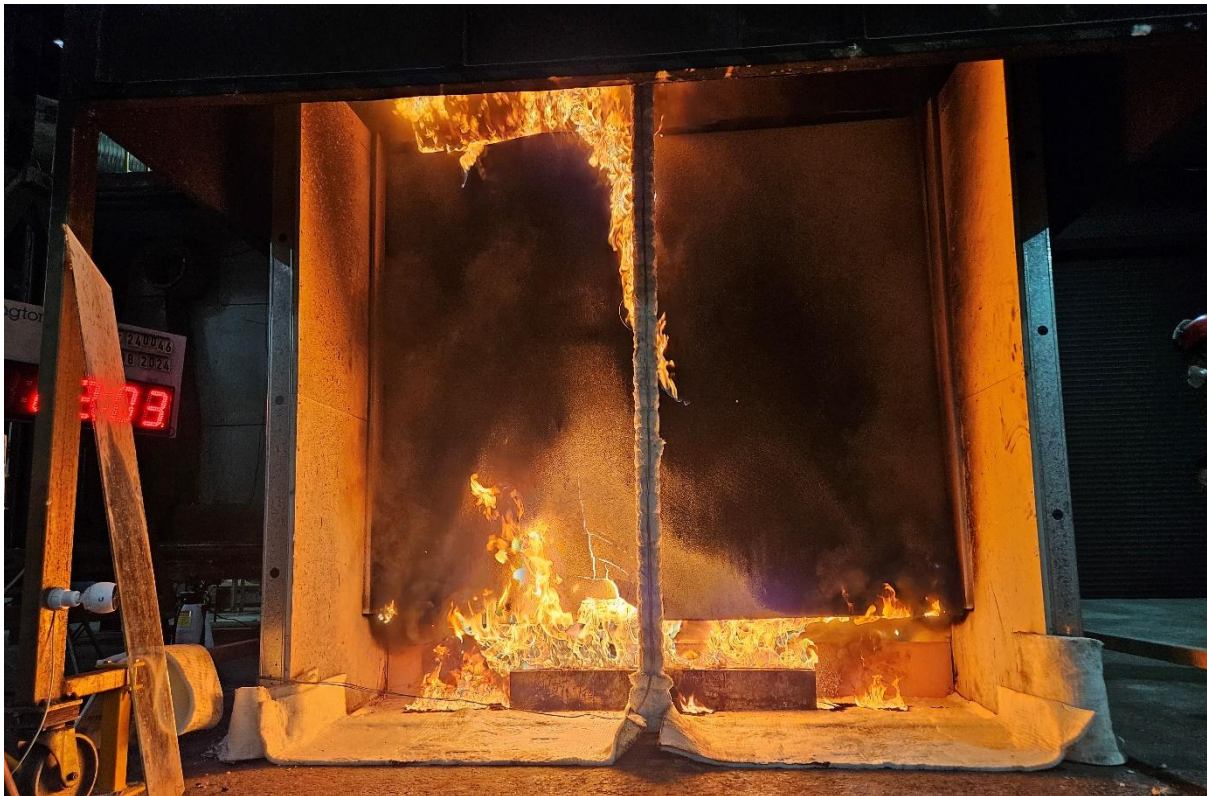
Figure 23 The specimen 22 minutes 3 seconds into the test (burner output at 300 kW)
