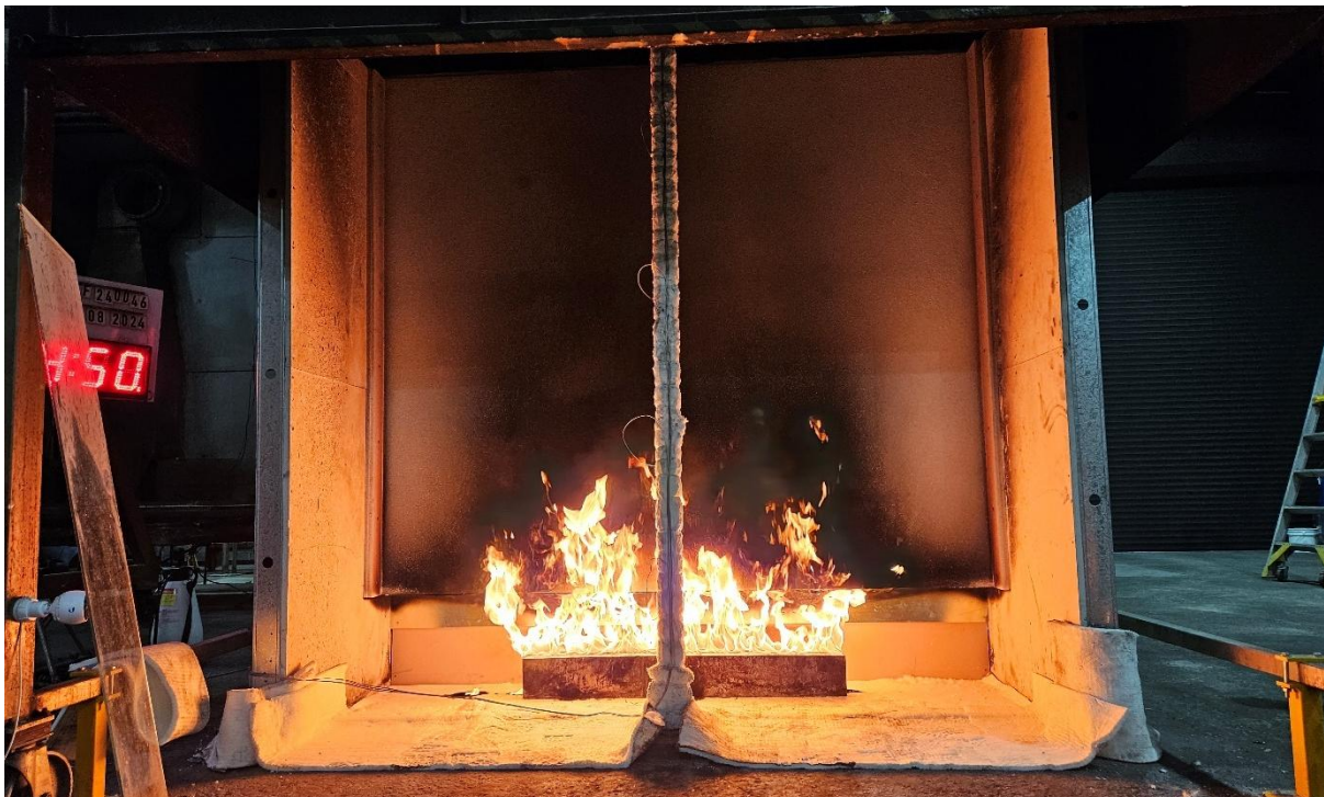
Figure 19 The specimen 14 minutes 50 seconds into the test (burner output at 100 kW)
