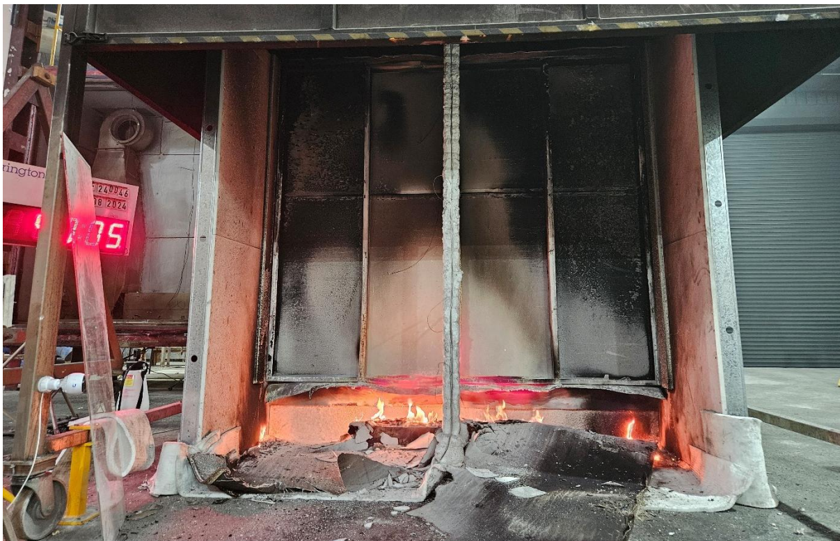
Figure 27 The specimen 40 minutes 5 seconds into the test (burner off)
