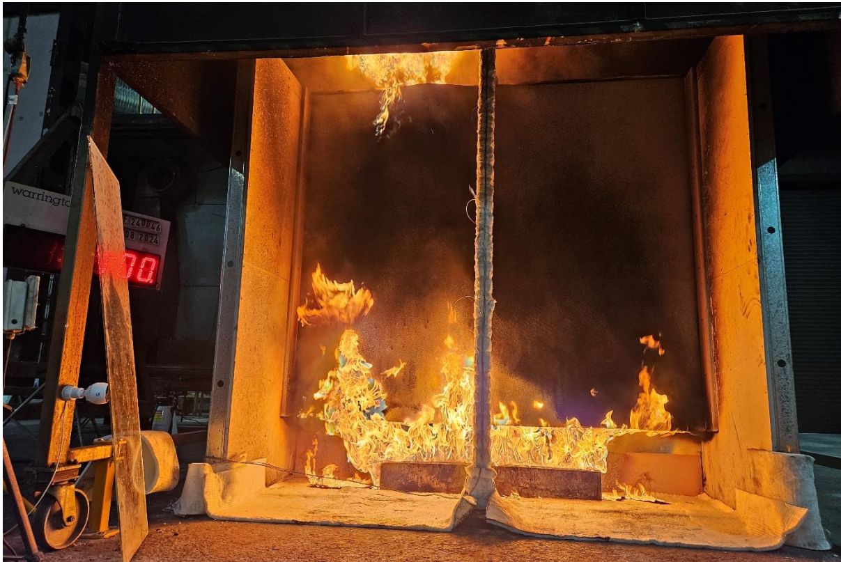
Figure 22 The specimen 21 minutes into the test (burner output at 300 kW)
