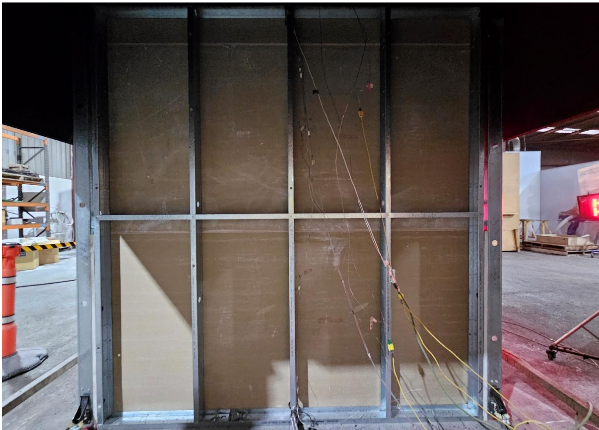
Figure 29 The specimen after the reaction to fire test – unexposed side
