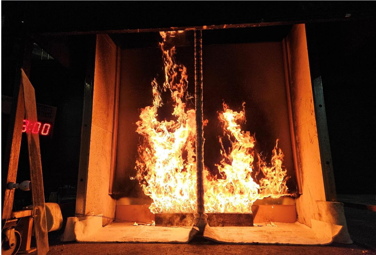
Figure 21 The specimen 18 minutes into the test (burner output at 300 kW)
