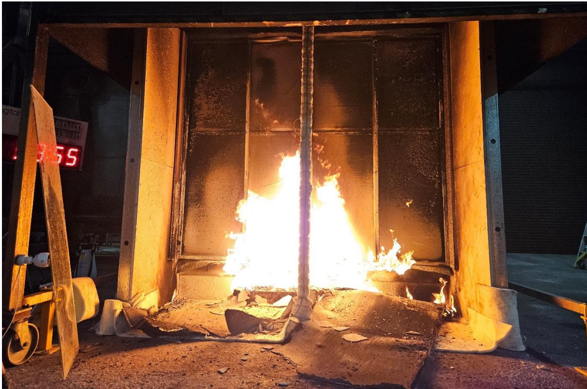
Figure 26 The specimen 39 minutes 55 seconds into the test (burner output at 300 kW)
