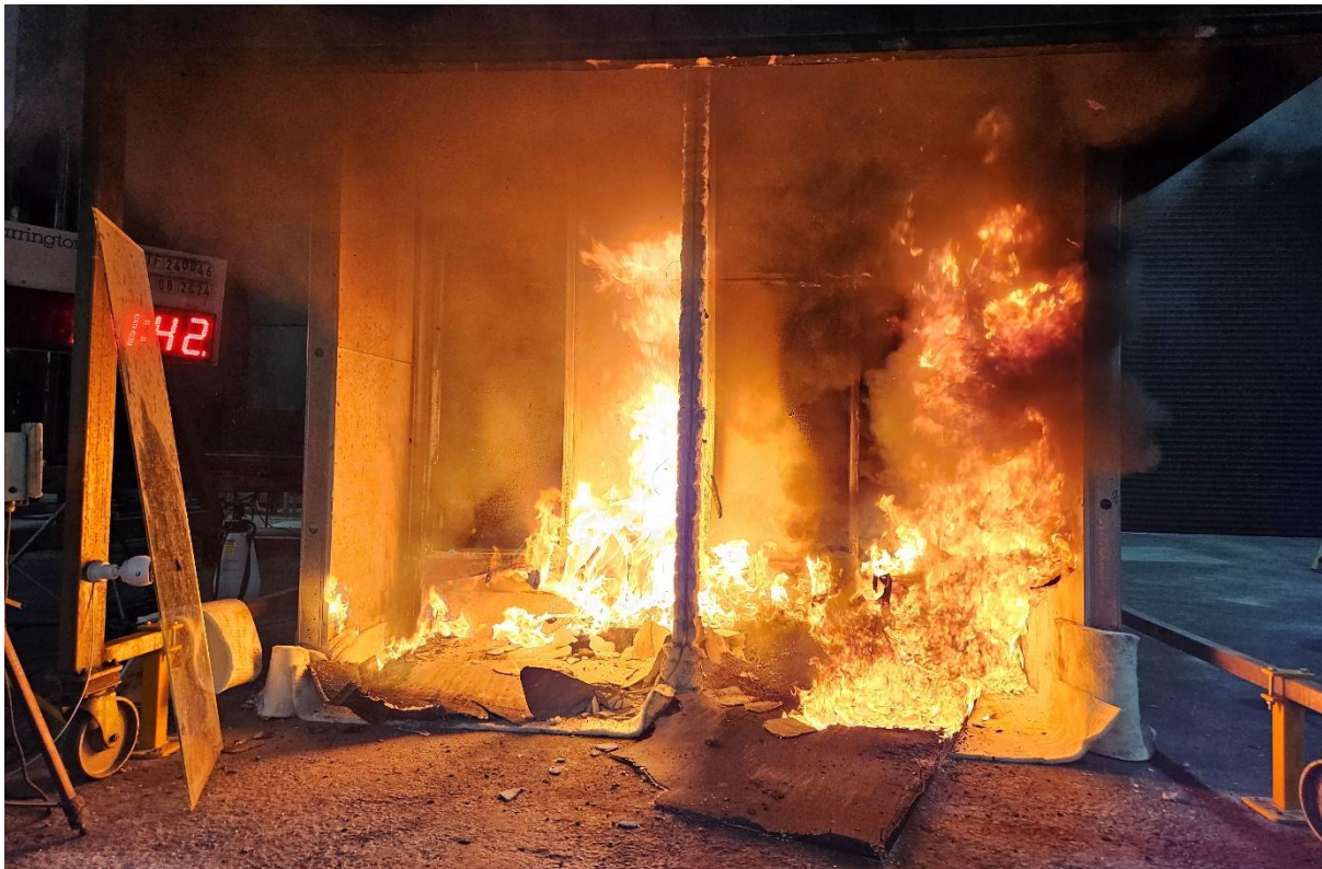
Figure 25 The specimen 31 minutes 42 seconds into the test (burner output at 300 kW)
