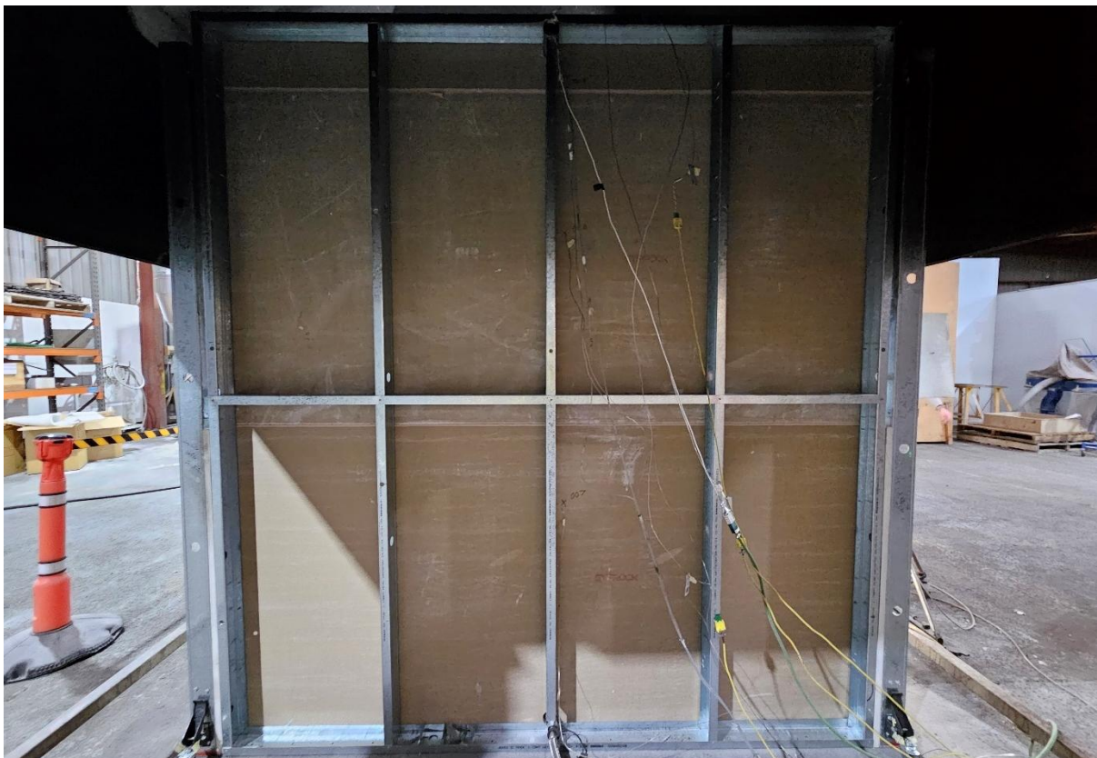
Figure 17 The specimen before the reaction to fire test – unexposed side
