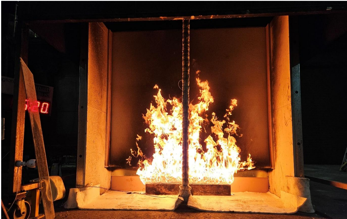
Figure 20 The specimen 15 minutes 20 seconds into the test (burner output at 300 kW)
