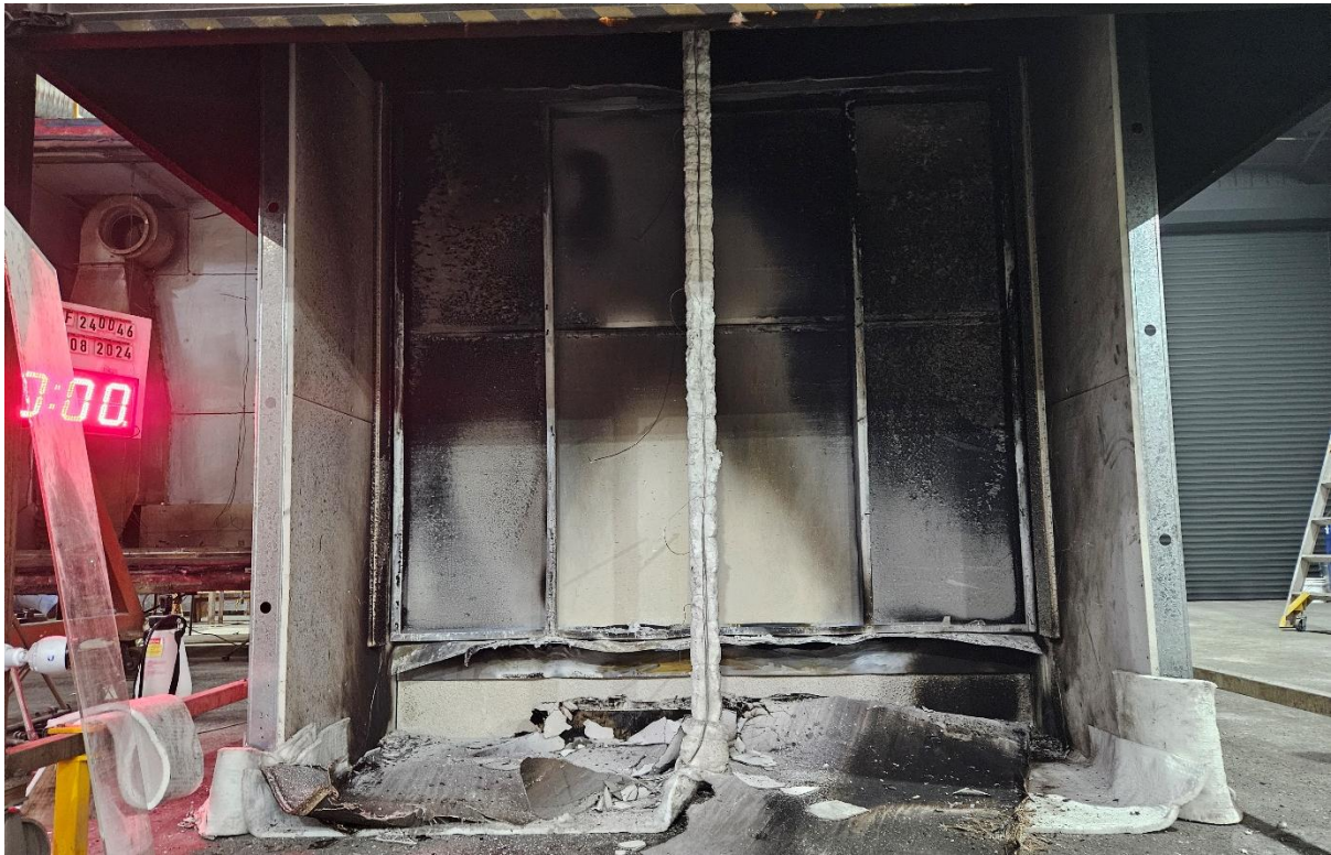
Figure 28 The specimen at end of the reaction to fire test – exposed side
