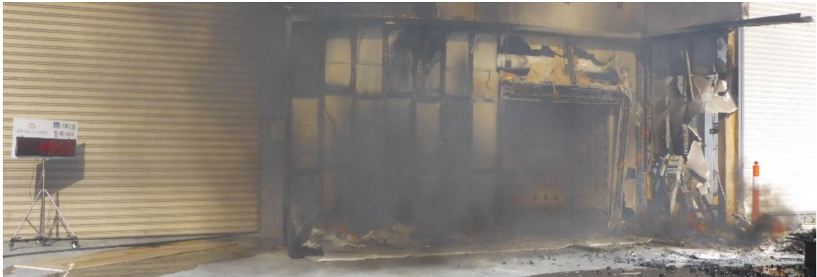
Figure 36 The wall system during the test – 49 minutes 55 seconds after crib ignition
