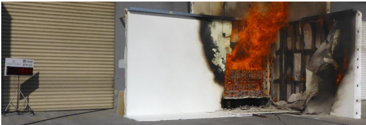
Figure 29 The wall system during the test – 19 minutes 54 seconds after crib ignition
