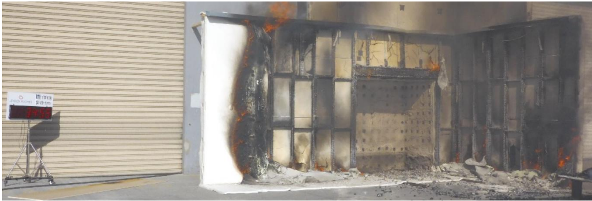
Figure 33 The wall system during the test – 34 minutes 55 seconds after crib ignition
