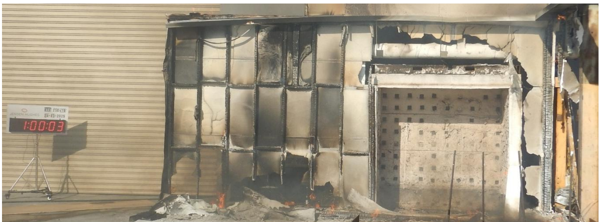
Figure 38 The wall system on completion of the test – main wall
