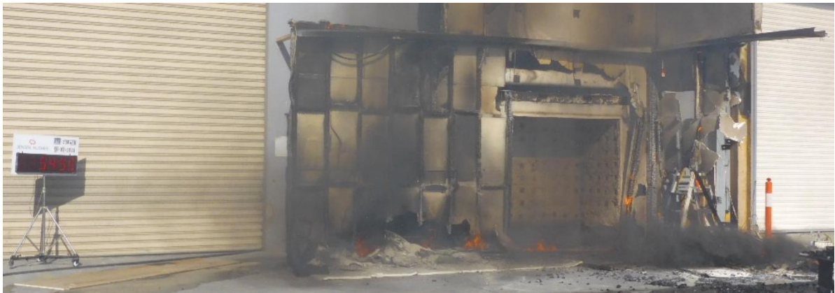
Figure 37 The wall system during the test – 54 minutes 55 seconds after crib ignition
