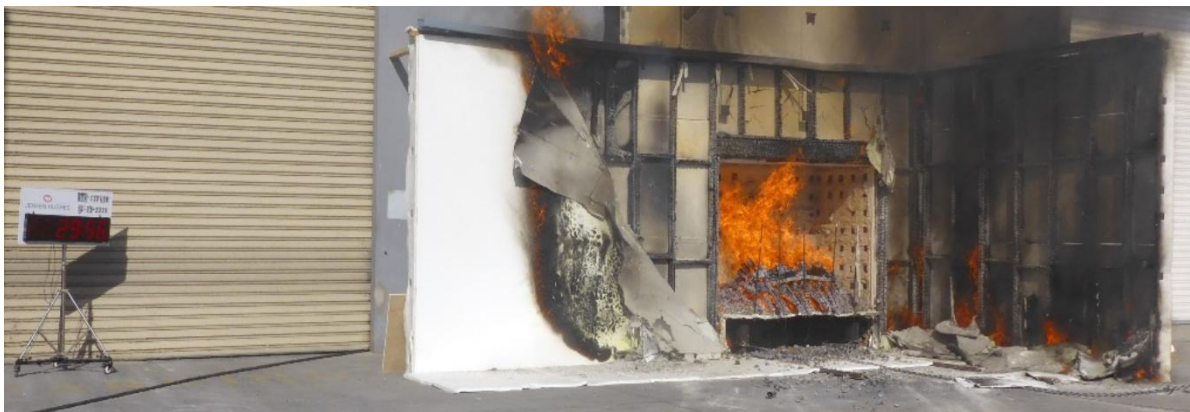
Figure 31 The wall system during the test – 29 minutes 55 seconds after crib ignition
