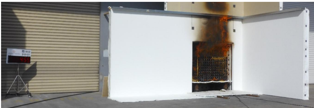
Figure 26 The wall system during the test – 4 minutes 55 seconds after crib ignition
