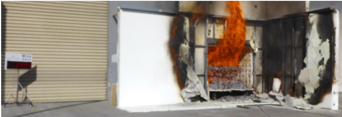
Figure 30 The wall system during the test – 24 minutes 54 seconds after crib ignition
