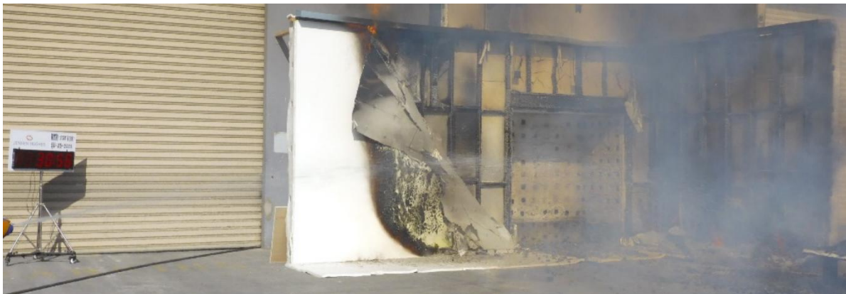
Figure 32 The wall system during the test – after removal of the crib, 30 minutes after ignition of crib
