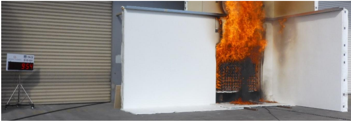
Figure 27 The wall system during the test – 9 minutes 54 seconds after crib ignition
