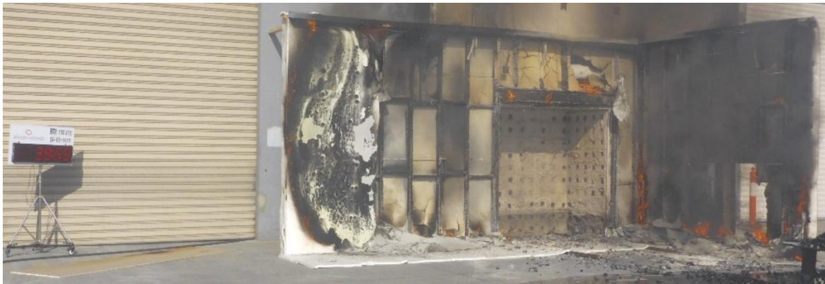
Figure 34 The wall system during the test – 39 minutes 55 seconds after crib ignition
