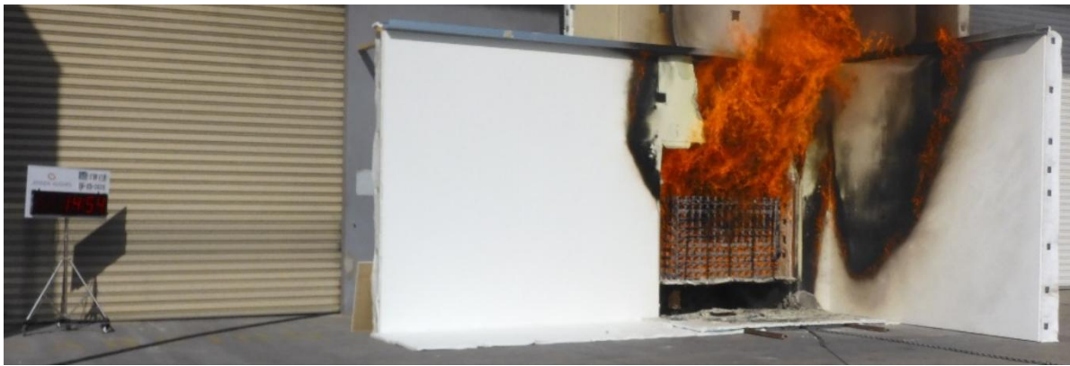
Figure 28 The wall system during the test – 14 minutes 54 seconds after crib ignition
