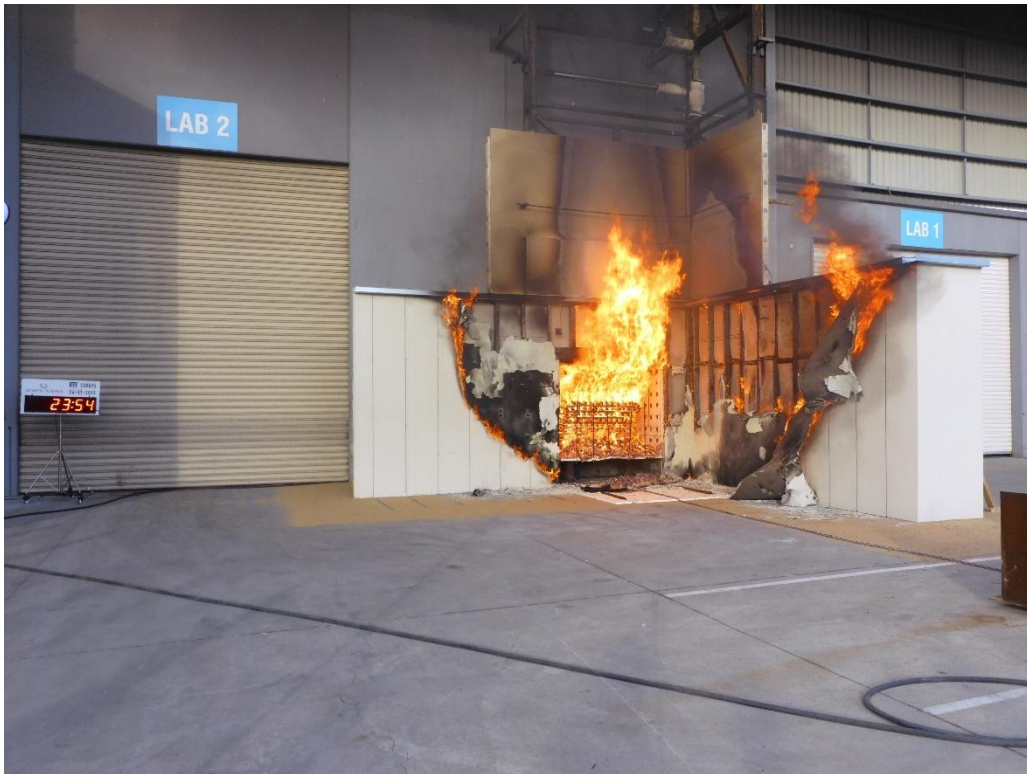
Figure 43 The wall system during the test – 23 minutes 54 seconds after crib ignition
