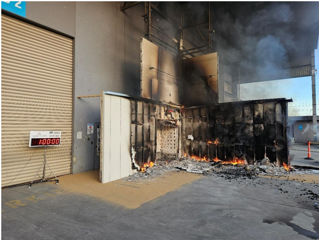
Figure 51 The wall system on completion of the test – exposed face
