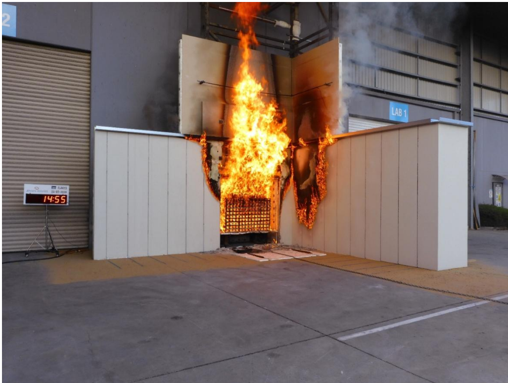
Figure 41 The wall system during the test – 14 minutes 55 seconds after crib ignition
