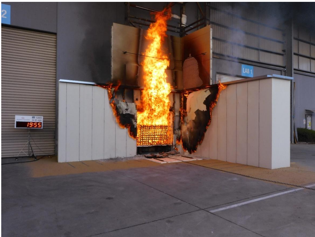
Figure 42 The wall system during the test – 19 minutes 55 seconds after crib ignition
