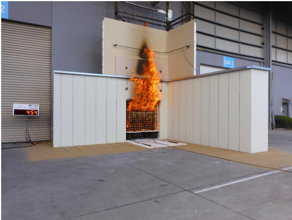
Figure 39 The wall system during the test – 4 minutes 54 seconds after crib ignition
