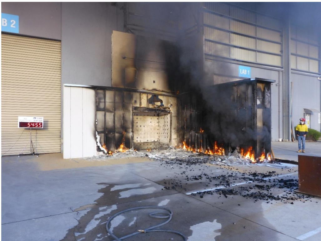
Figure 50 The wall system during the test – 54 minutes 55 seconds after crib ignition
