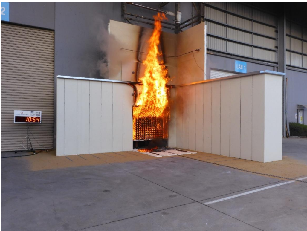
Figure 40 The wall system during the test – 10 minutes 54 seconds after crib ignition
