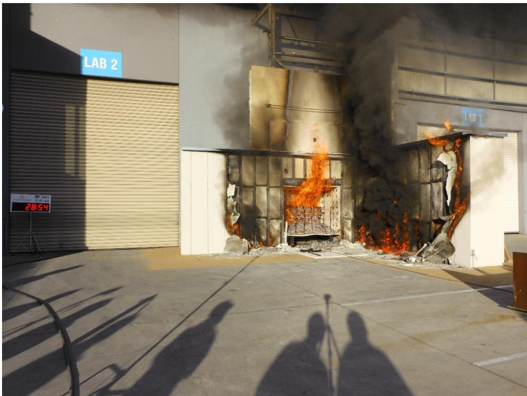
Figure 44 The wall system during the test – 28 minutes 54 seconds after crib ignition
