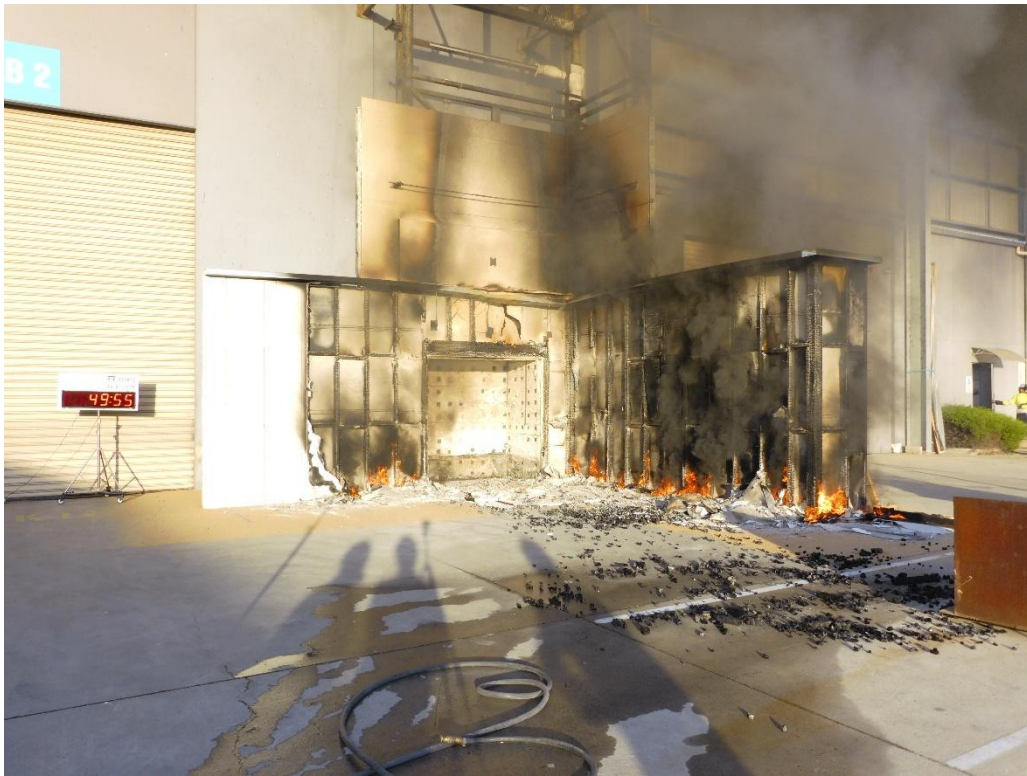
Figure 49 The wall system during the test – 49 minutes 55 seconds after crib ignition
