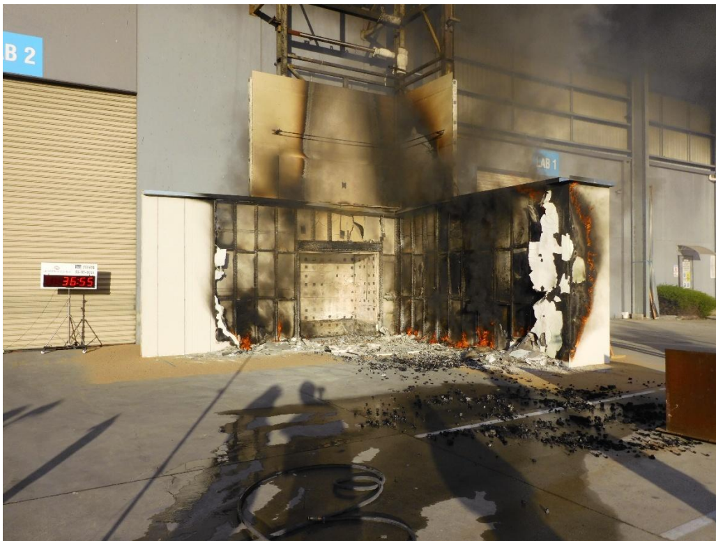
Figure 46 The wall system during the test – 36 minutes 55 seconds after crib ignition
