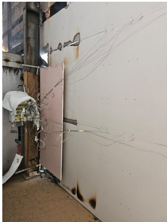
Figure 52 The wall system on completion of the test – unexposed main wall face
