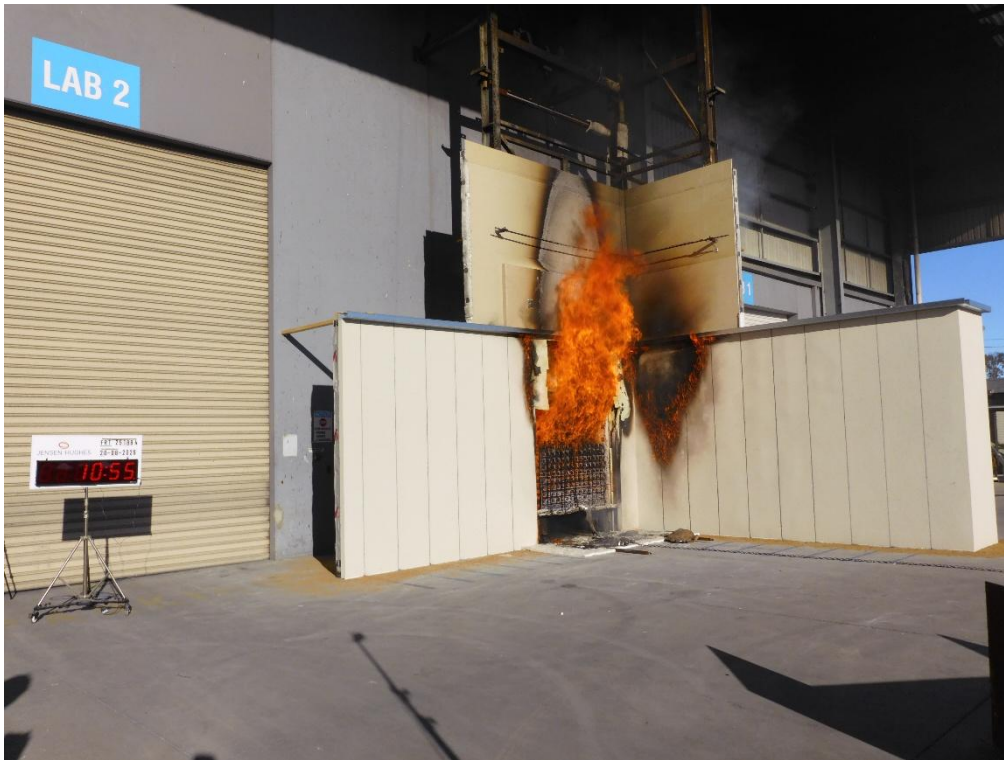
Figure 41 The wall system during the test – 10 minutes 55 seconds after crib ignition
