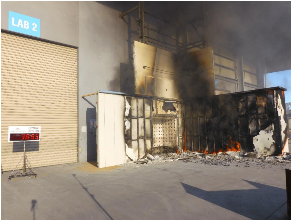
Figure 47 The wall system during the test – 36 minutes 55 seconds after crib ignition
