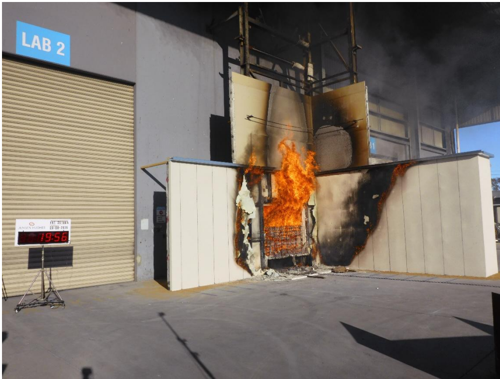
Figure 43 The wall system during the test – 19 minutes 56 seconds after crib ignition
