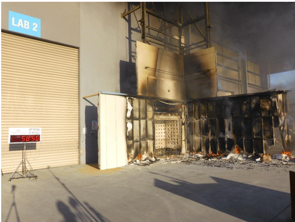
Figure 52 The wall system during the test – 58 minutes 56 seconds after crib ignition
