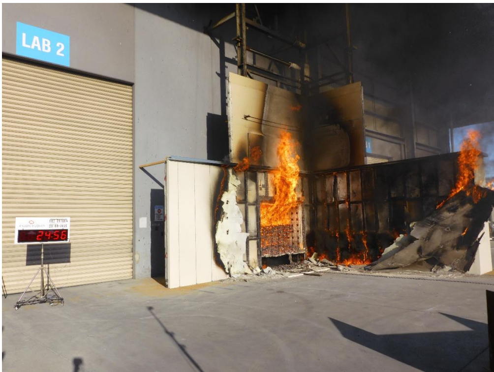
Figure 44 The wall system during the test – 24 minutes 56 seconds after crib ignition
