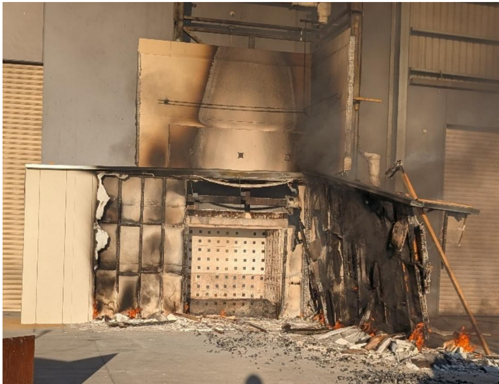
Figure 53 The wall system on completion of the test – exposed face
