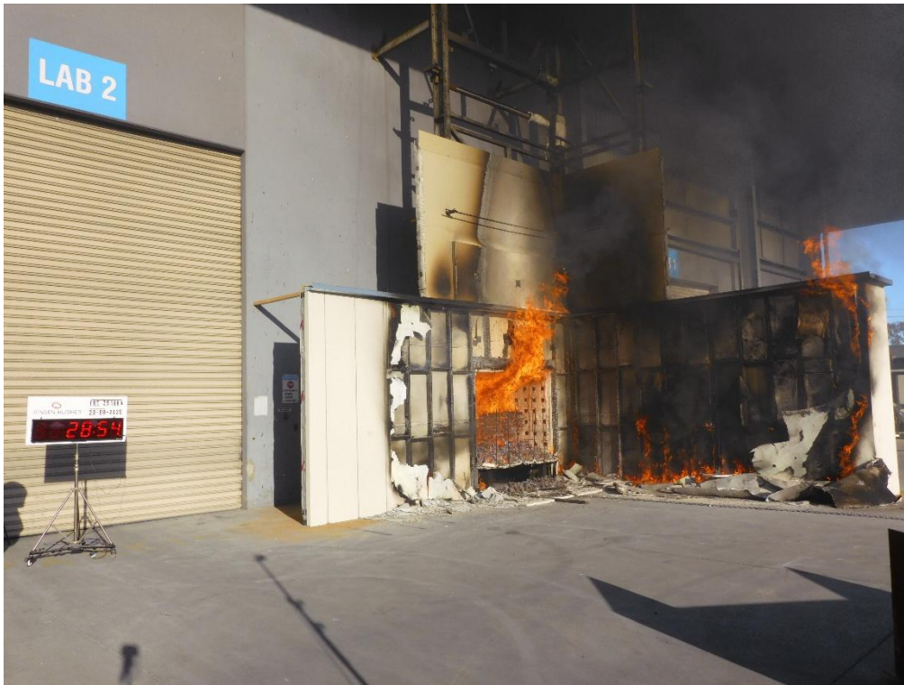
Figure 45 The wall system during the test – 28 minutes 54 seconds after crib ignition
