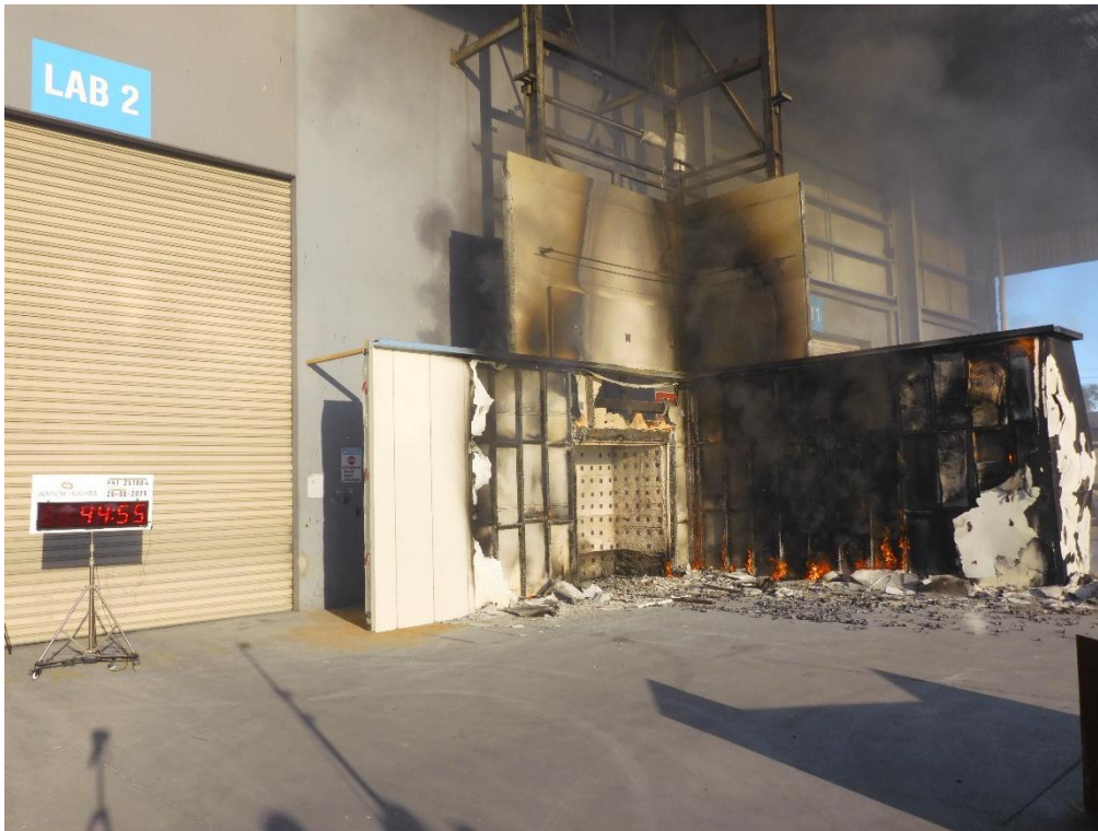
Figure 49 The wall system during the test – 44 minutes 55 seconds after crib ignition
