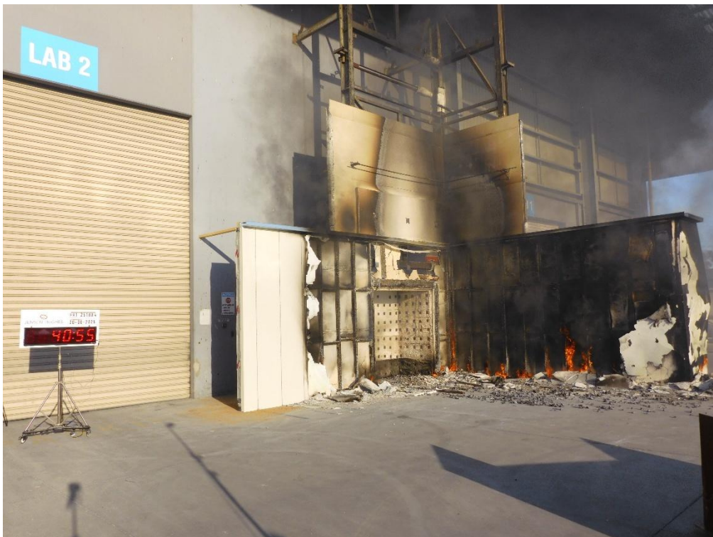
Figure 48 The wall system during the test – 40 minutes 55 seconds after crib ignition
