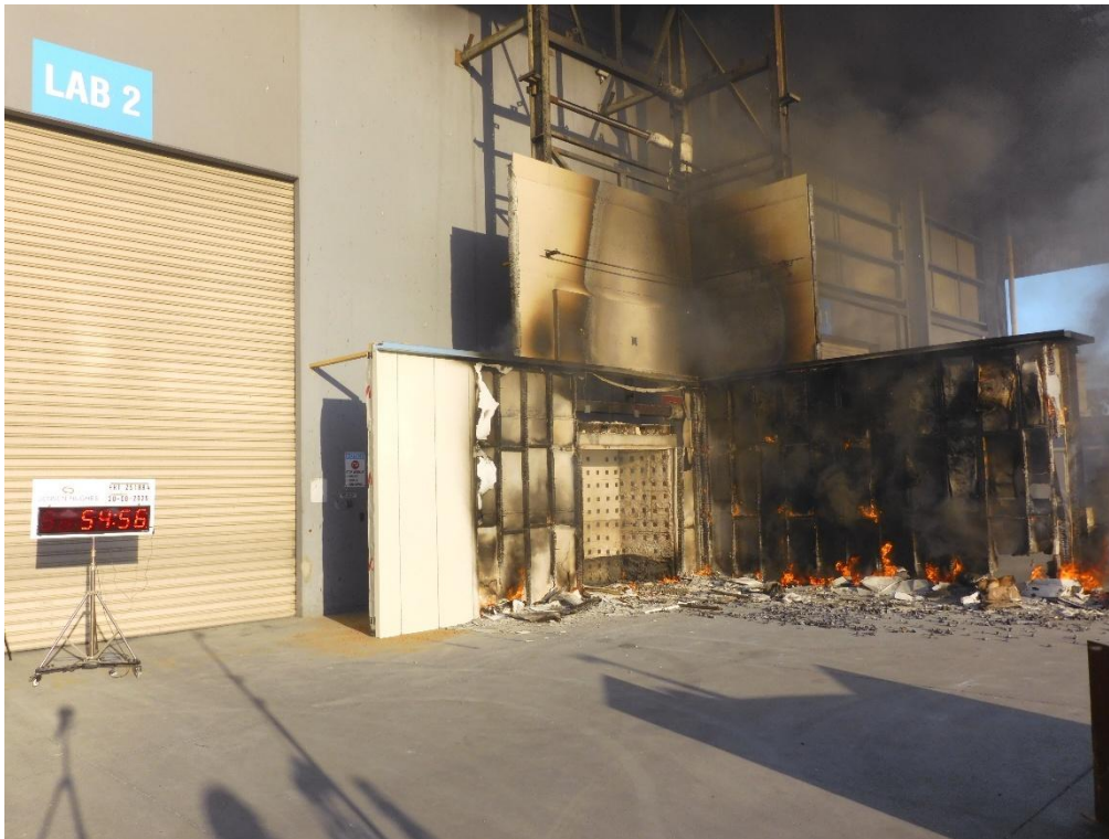
Figure 51 The wall system during the test – 54 minutes 56 seconds after crib ignition
