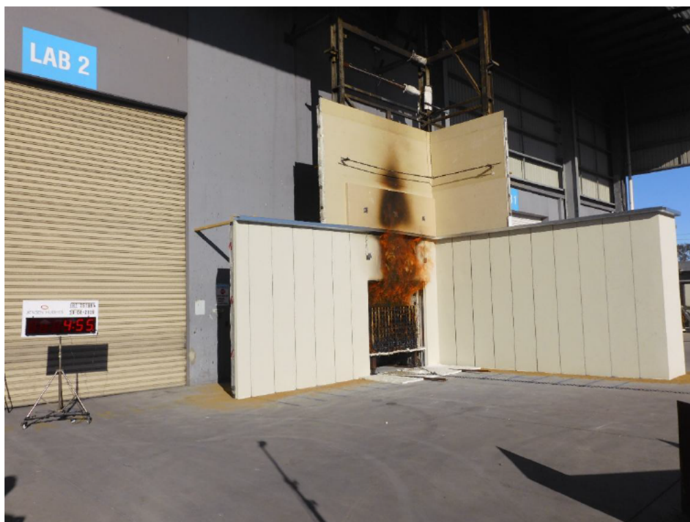
Figure 40 The wall system during the test – 4 minutes 55 seconds after crib ignition
