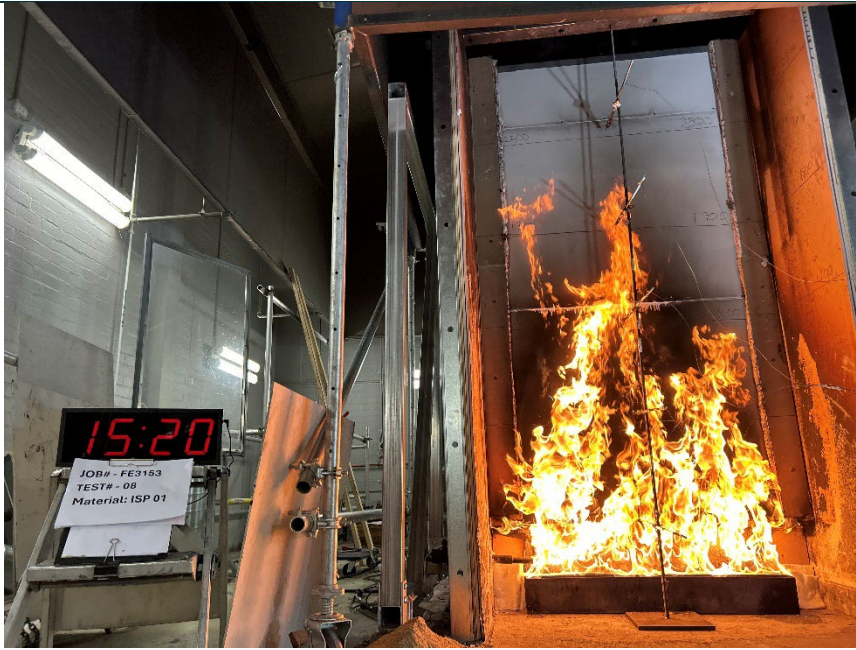
Test 8 – ISP-01 PIR with steel capping
