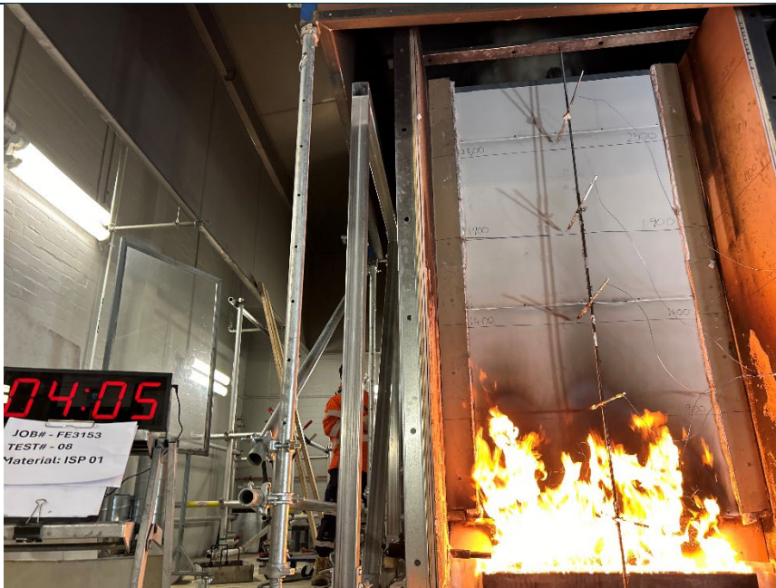
Test 8 – ISP-01 PIR with steel capping
