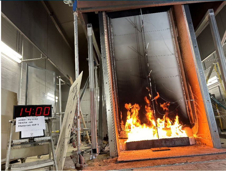
Test 6, ISP-01 PIR, No steel capping
