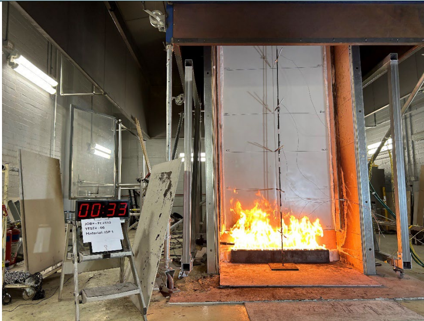
Test 6, ISP-01 PIR, No steel capping
