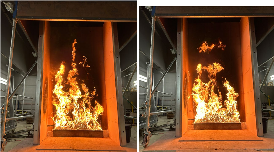
Figure 15. Burner at 300 kW.
