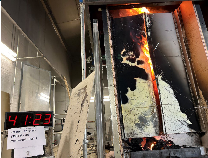
Test 6, ISP-01 PIR, No steel capping
