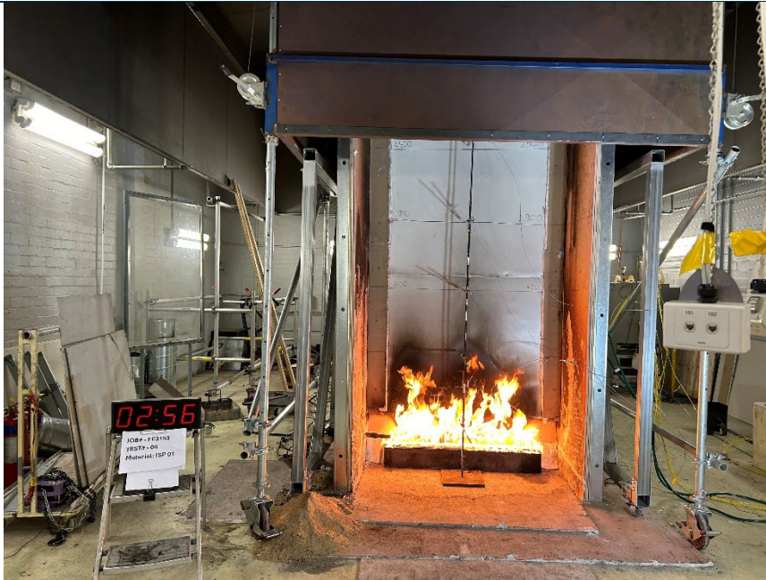
Test 8 – ISP-01 PIR with steel capping
