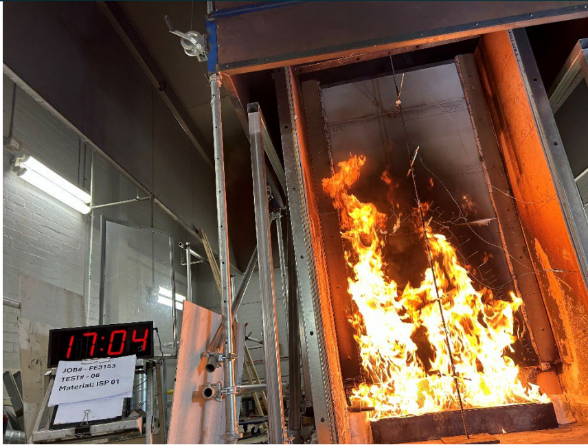
Test 8 – ISP-01 PIR with steel capping
