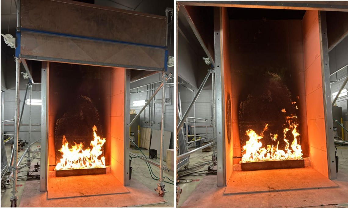
Figure 14. Burner at 100 kW.
