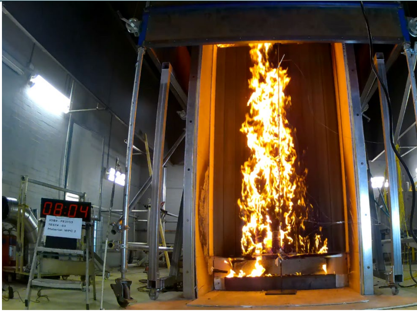
Test 3, WPC-02, at 484s, Burner turned off just prior to suppression with fire hose reel.
