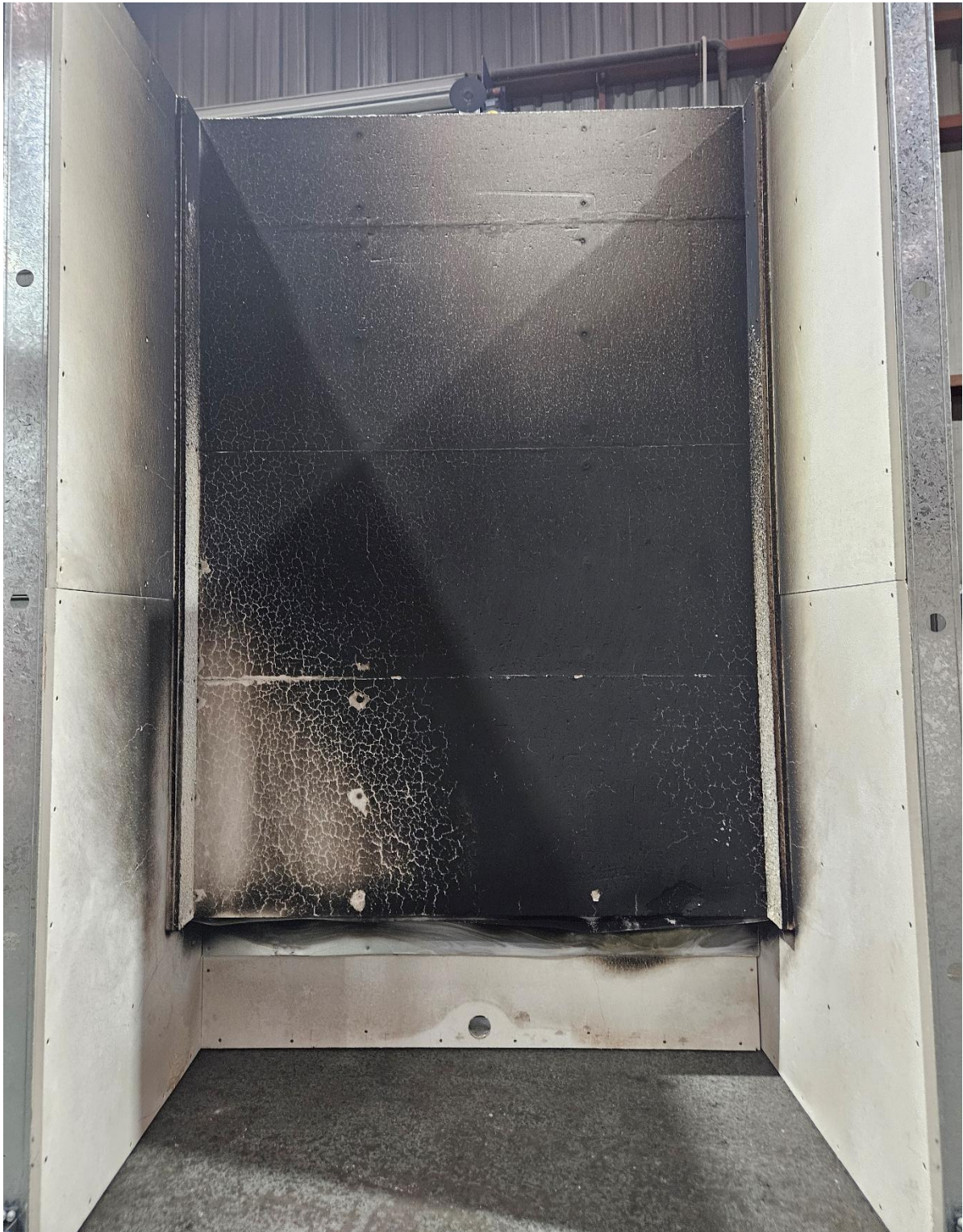
Figure 25 The specimen at end of the reaction to fire test – exposed side
