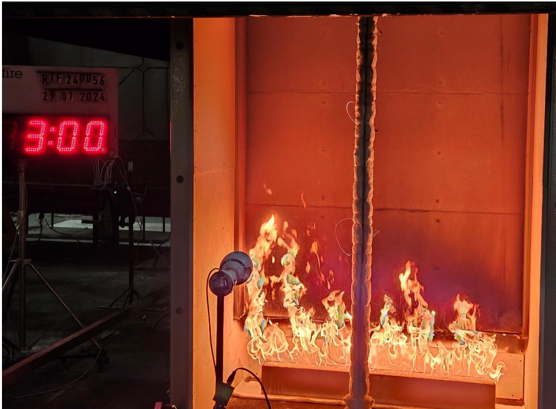
Figure 17 The specimen 3 minutes into the test (burner output at 100 kW)
