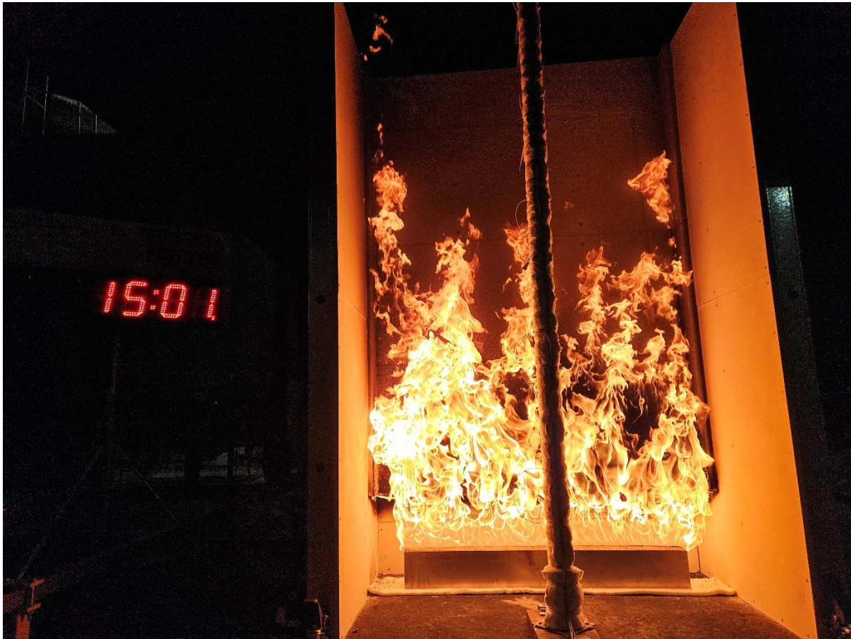
Figure 20 The specimen 15 minutes 01 seconds into the test (burner output at 300 kW)
