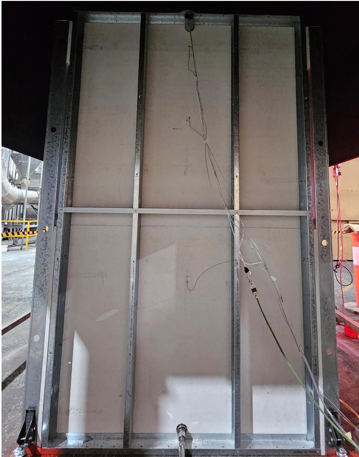
Figure 16 The specimen before the reaction to fire test – unexposed side
