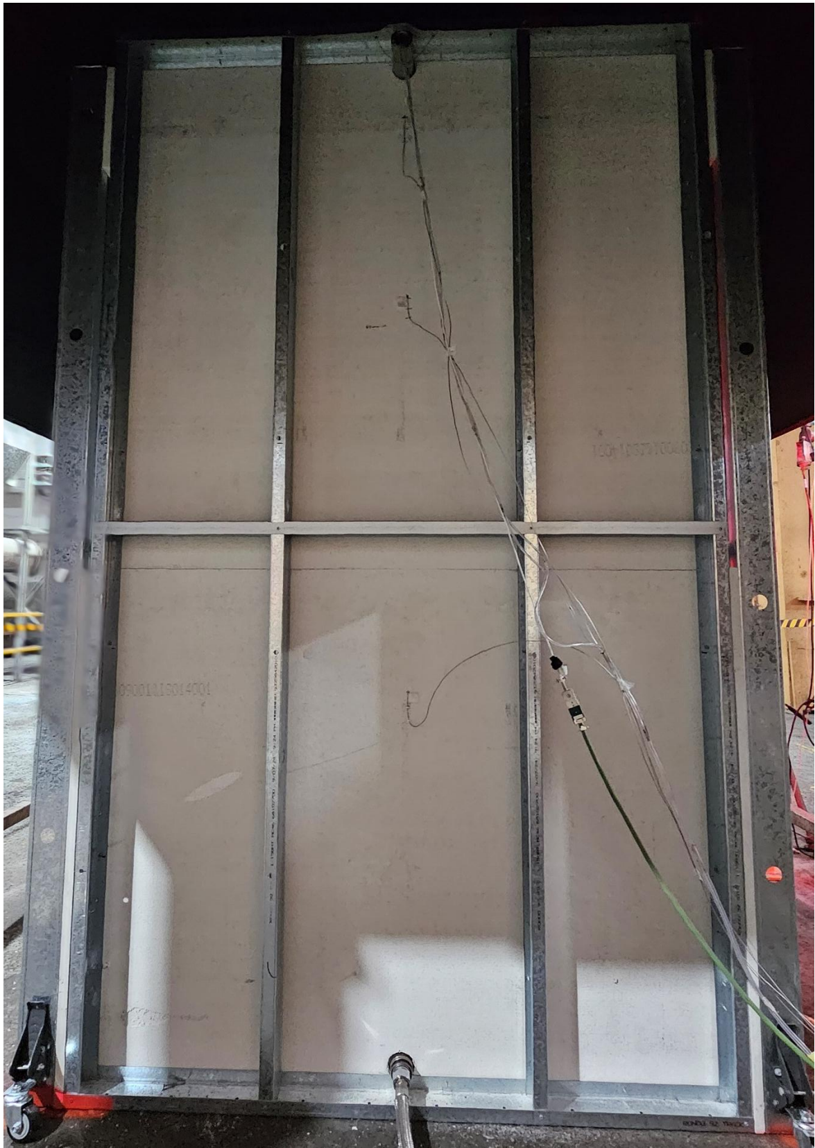
Figure 26 The specimen after the reaction to fire test – unexposed side
