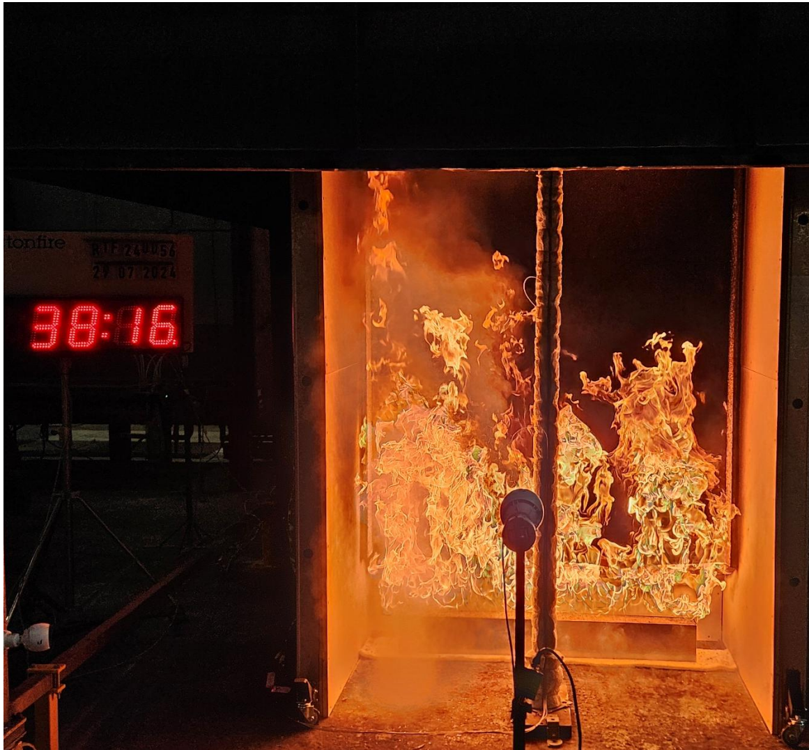
Figure 22 The specimen 38 minutes 16 seconds into the test (burner output at 300 kW)
