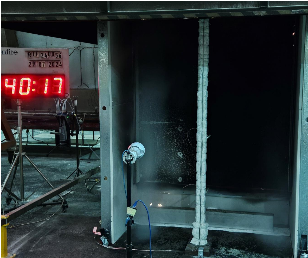
Figure 23 The specimen 40 minutes 17 seconds into the test (burner off)
