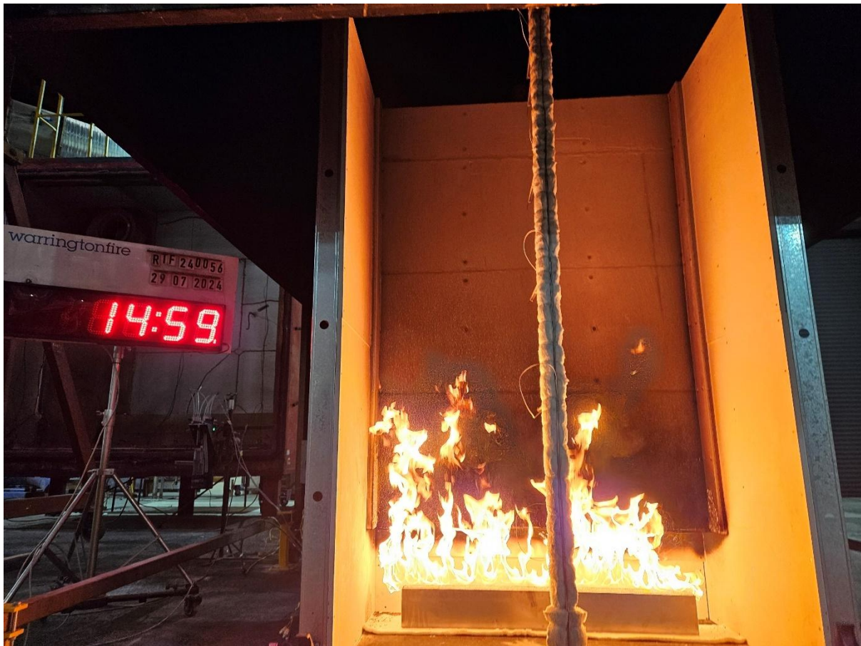
Figure 19 The specimen 14 minutes 59 seconds into the test (burner output at 100 kW)
