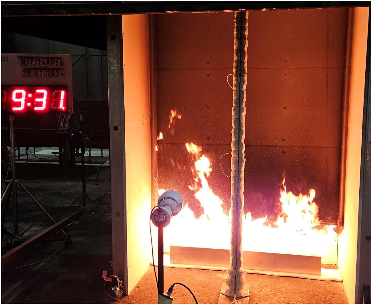
Figure 18 The specimen 9 minutes 31 seconds into the test (burner output at 100 kW)
