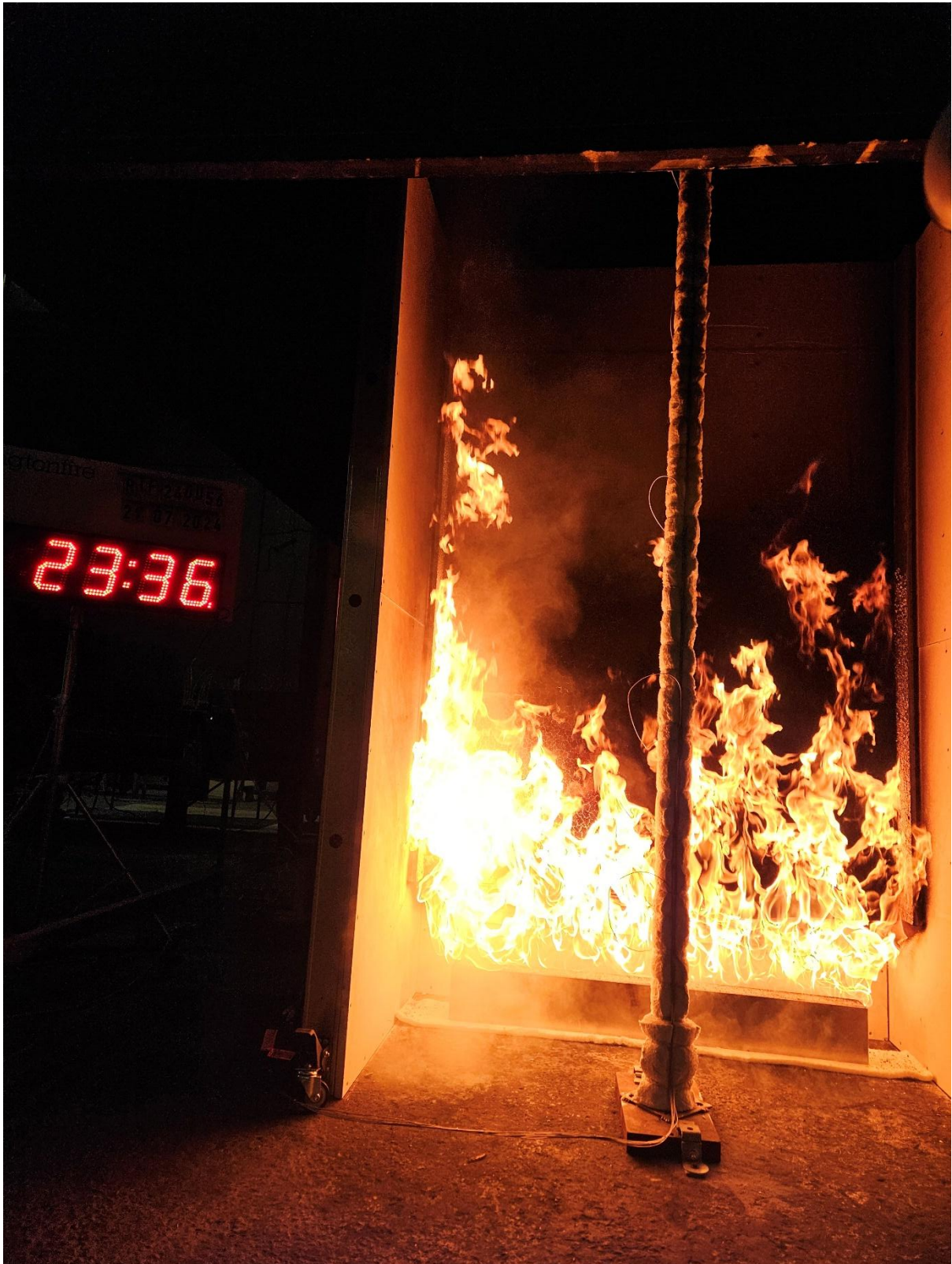
Figure 21 The specimen 23 minutes 36 seconds into the test (burner output at 300 kW)
