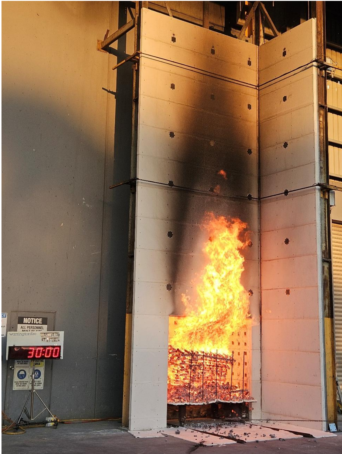
Figure 22 The external wall system during the test – specimen during removal of the crib, 30 minutes after ignition of crib
