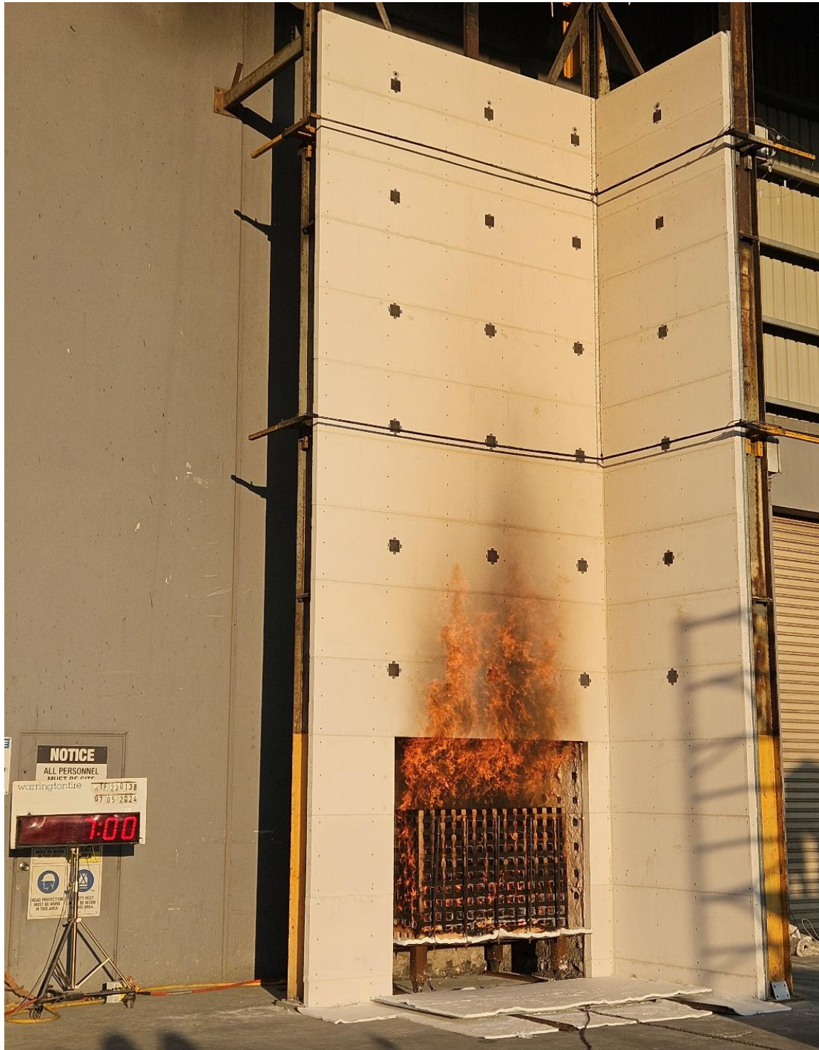
Figure 20 The external wall system during the test – 7 minutes after crib ignition
