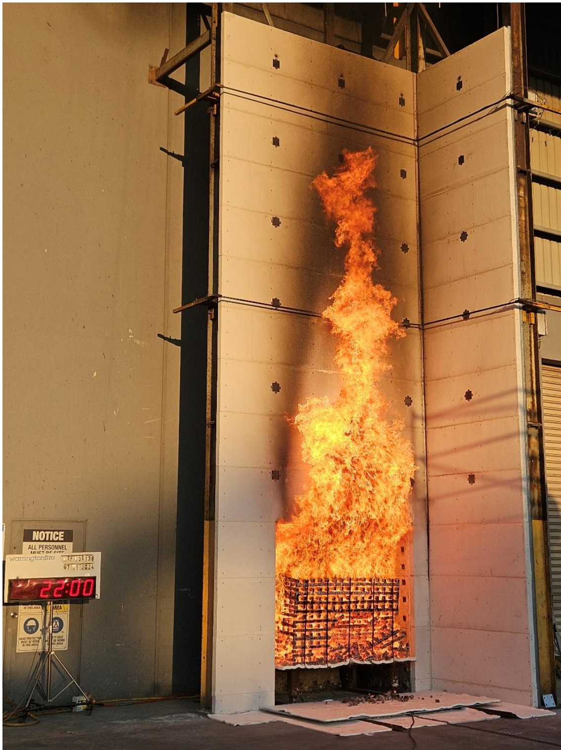
Figure 21 The external wall system during the test – 22 minutes after crib ignition
