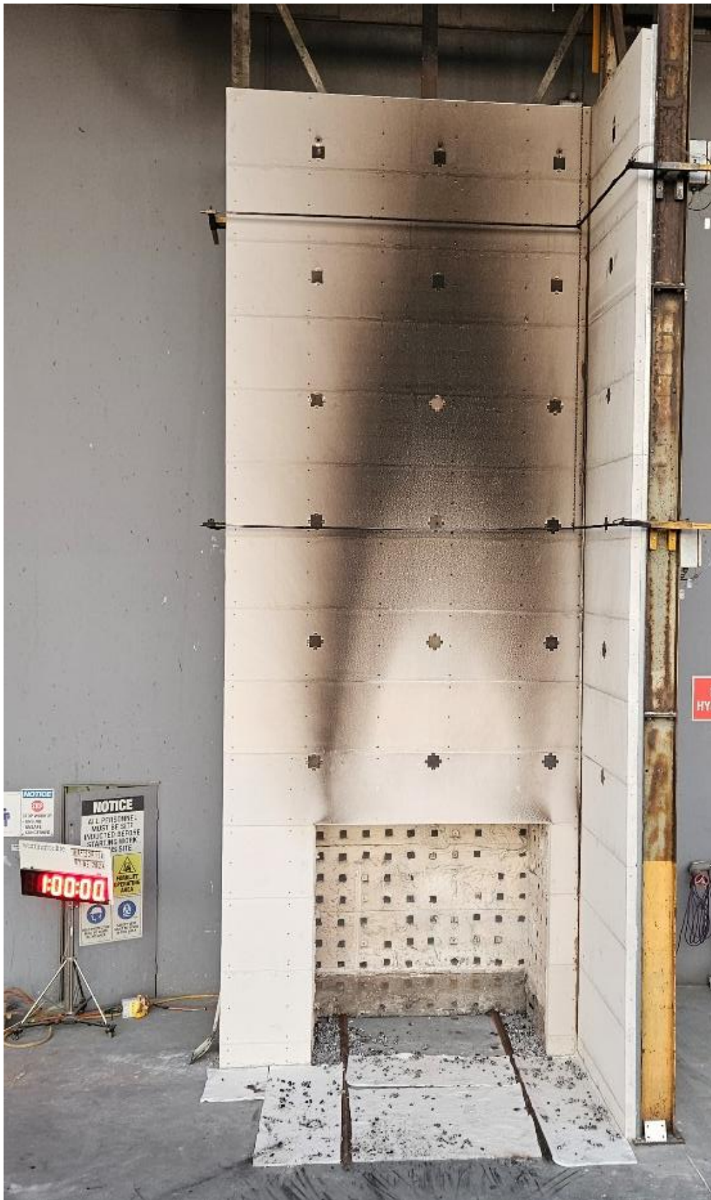
Figure 24 The external wall system on completion of the test – main wall
