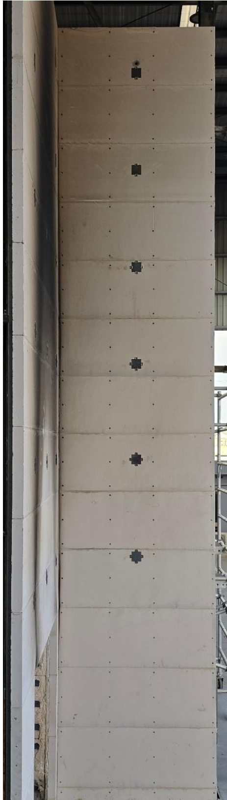
Figure 25 The external wall system on completion of the test – wing wall
